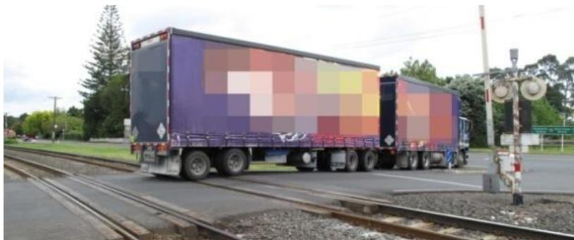
A total of 362 level crossings with short stacking distances are rated as high risk.<sup>2</sup> At level crossings with a short stacking distance, a long vehicle, even though it complies with road regulations, is unable to clear the level crossing when
