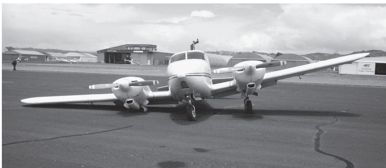
Landing gear collapse after landing in an older aeroplane
