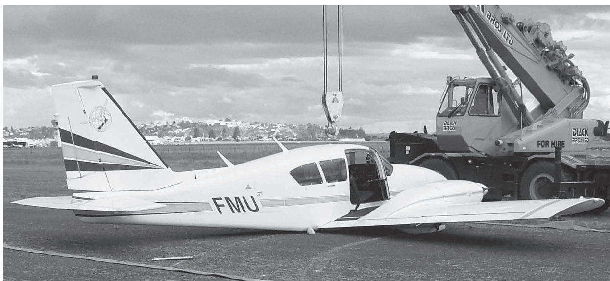
ZK-FMU with failed landing gear
