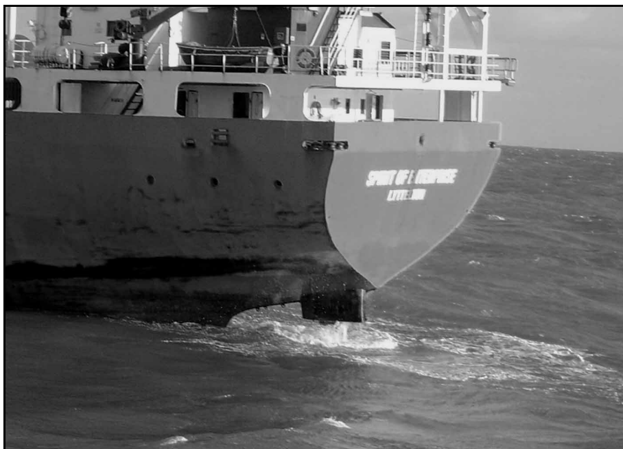
Container ship Spirit of Enterprise , touching bottom and loss of rudder, Manukau Bar, 16 August 2003 (Investigation 03-212, published in 2003/2004 year)
