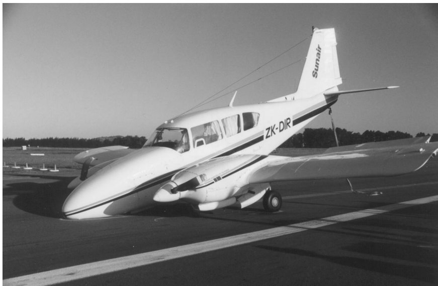
Piper PA23 Aztec, ZK-DIR, nose undercarriage collapse after landing, Gisborne Aerodrome, 14 December 2000 (investigation 00-014). There were no injuries.
