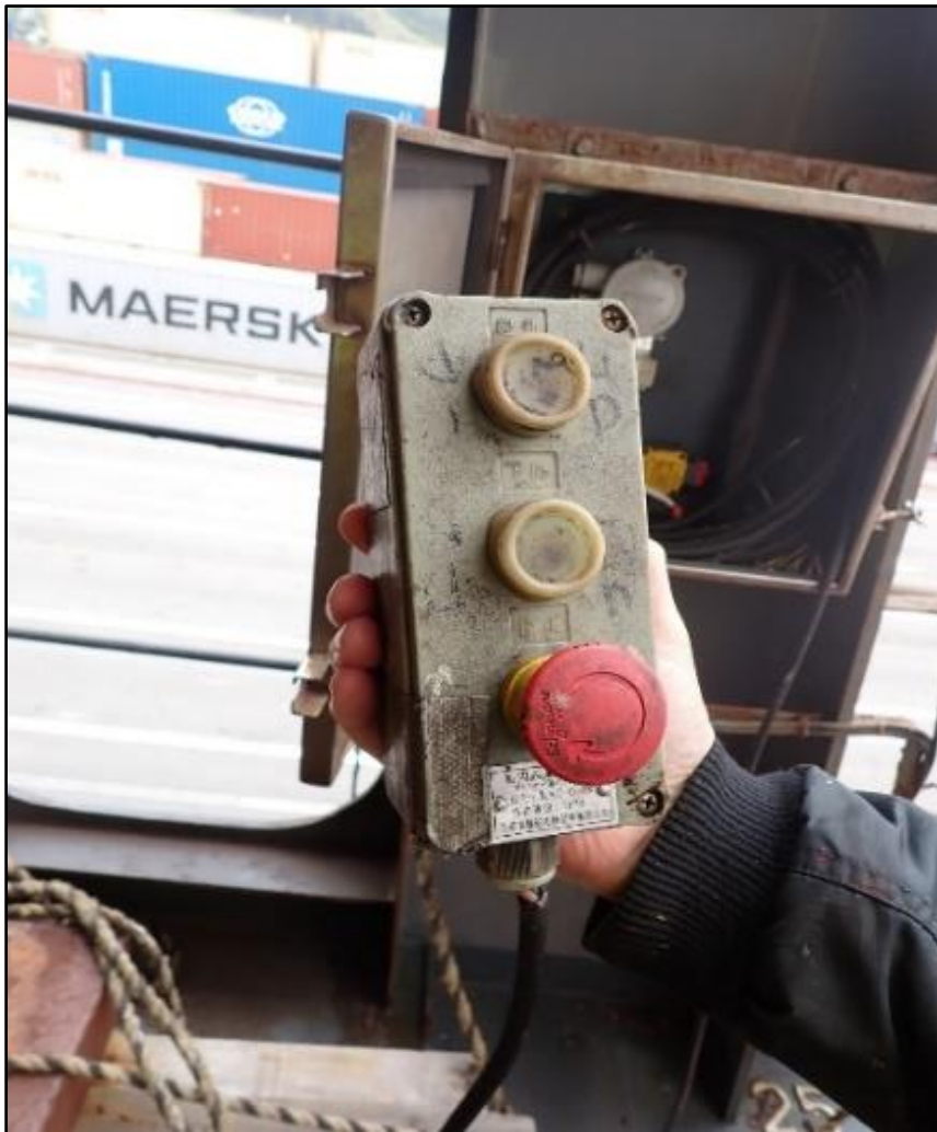
Figure 4: Accommodation ladder remote control
