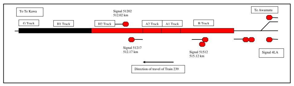
Figure 6 Track indications as Train 239 occupied H2 Track
