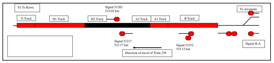
Figure 9 Track indications as Train 239 occupied G Track and vacated H2 Track
