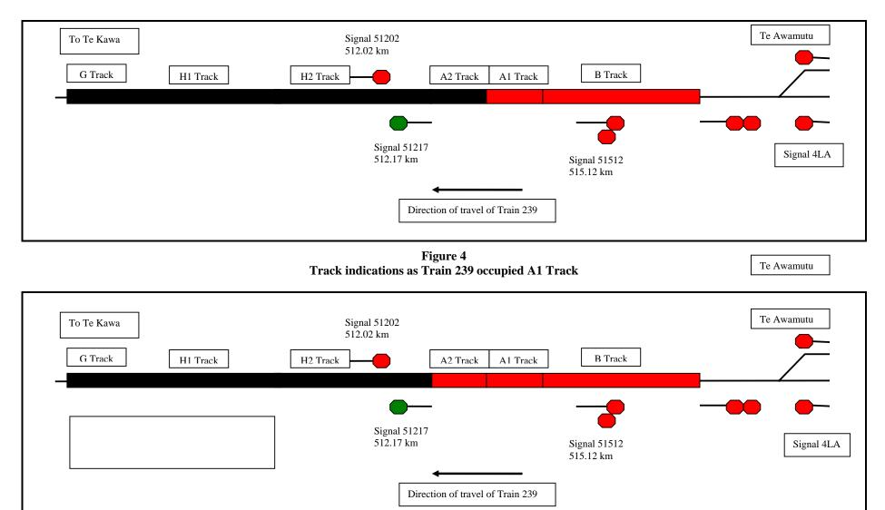
Figure 5 Track indications as Train 239 occupied A2 Track
