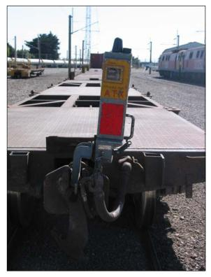
Figure 10 Trainlink ATX train end monitor attached to the wagon coupling
