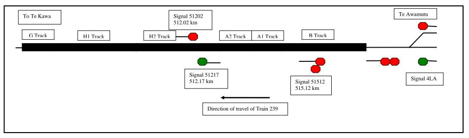
Figure 2 Track indications prior to departure of Train 239 from Te Awamutu
