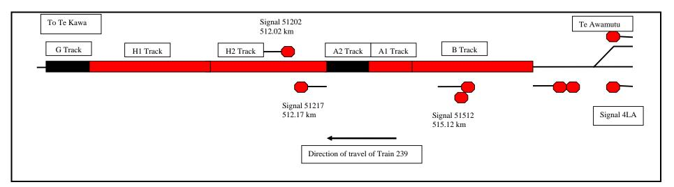
Figure 8 Track indications as Train 239 occupied H1 Track
