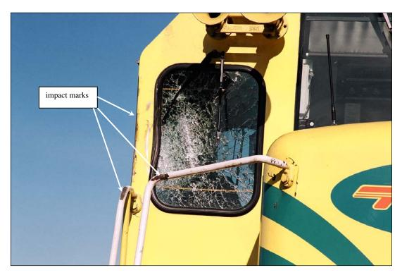
Figure 4 Locomotive cab forward window of MP2 after impact (photo courtesy New Zealand Police)
