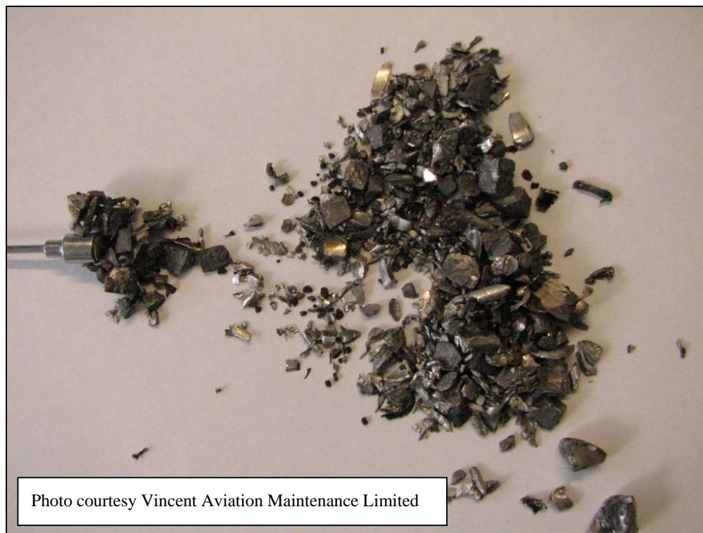
Figure 2 Debris from oil suction screen, with small test magnet at left
