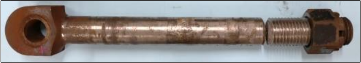
Figure 8: Broken tailpin from carriage one
