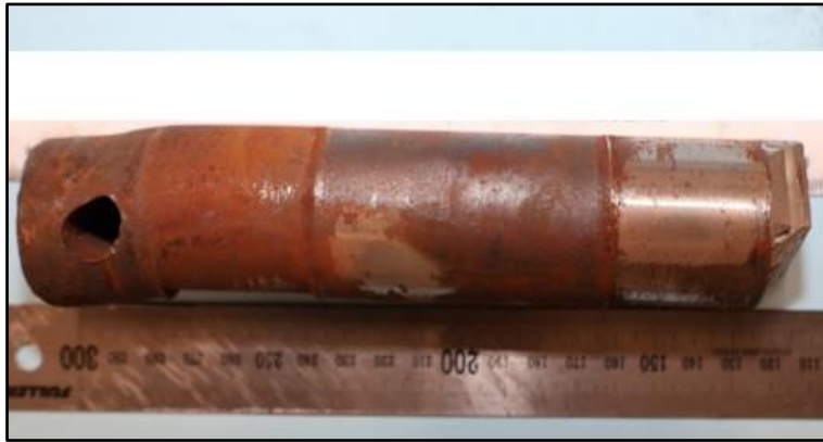
Figure 22: Drawbar pin from AKS coupler that parted
