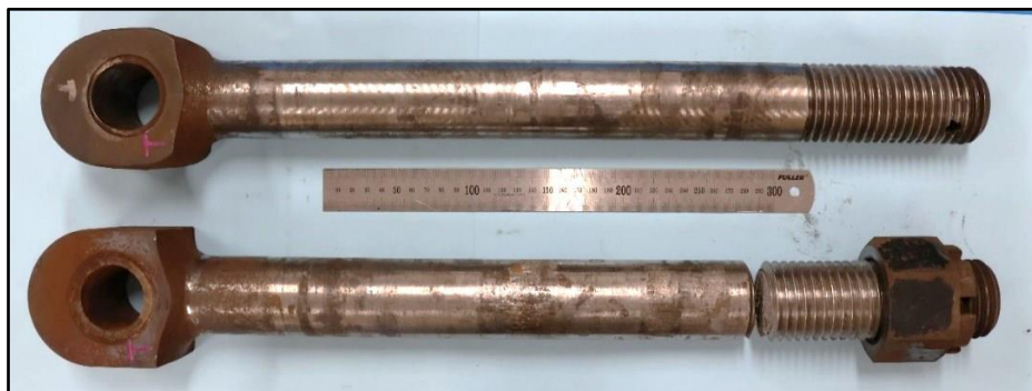
Figure 19: Tailpins from each end of carriage one
