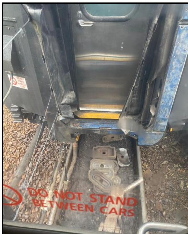
Figure 11: Parted gap between first and second carriages (Credit KiwiRail)
