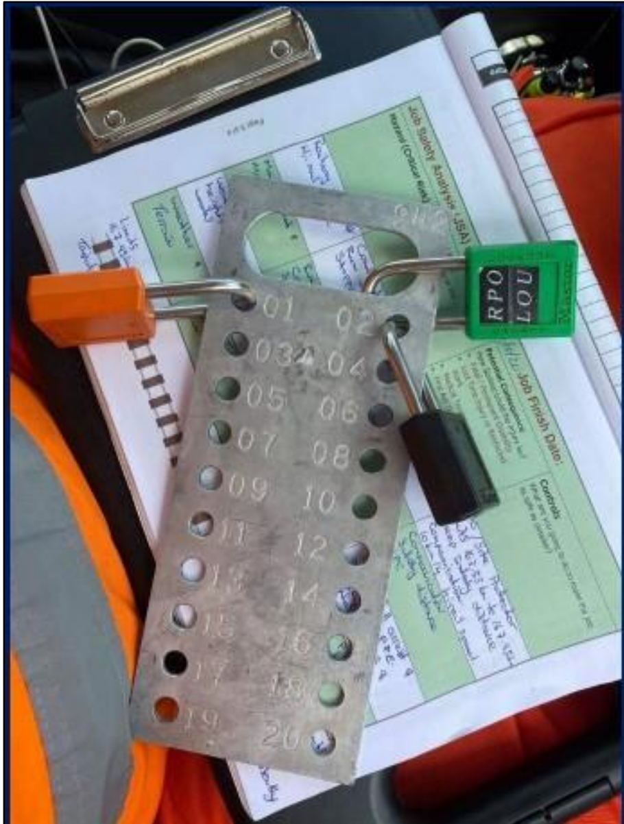
Figure 7: KiwiRail frame and padlock system
