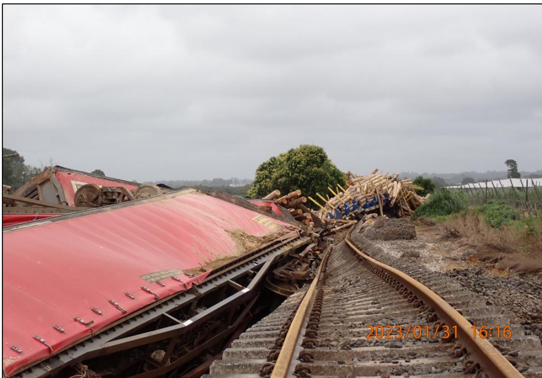
Figure 13: Derailed wagons and washed-out track formation
