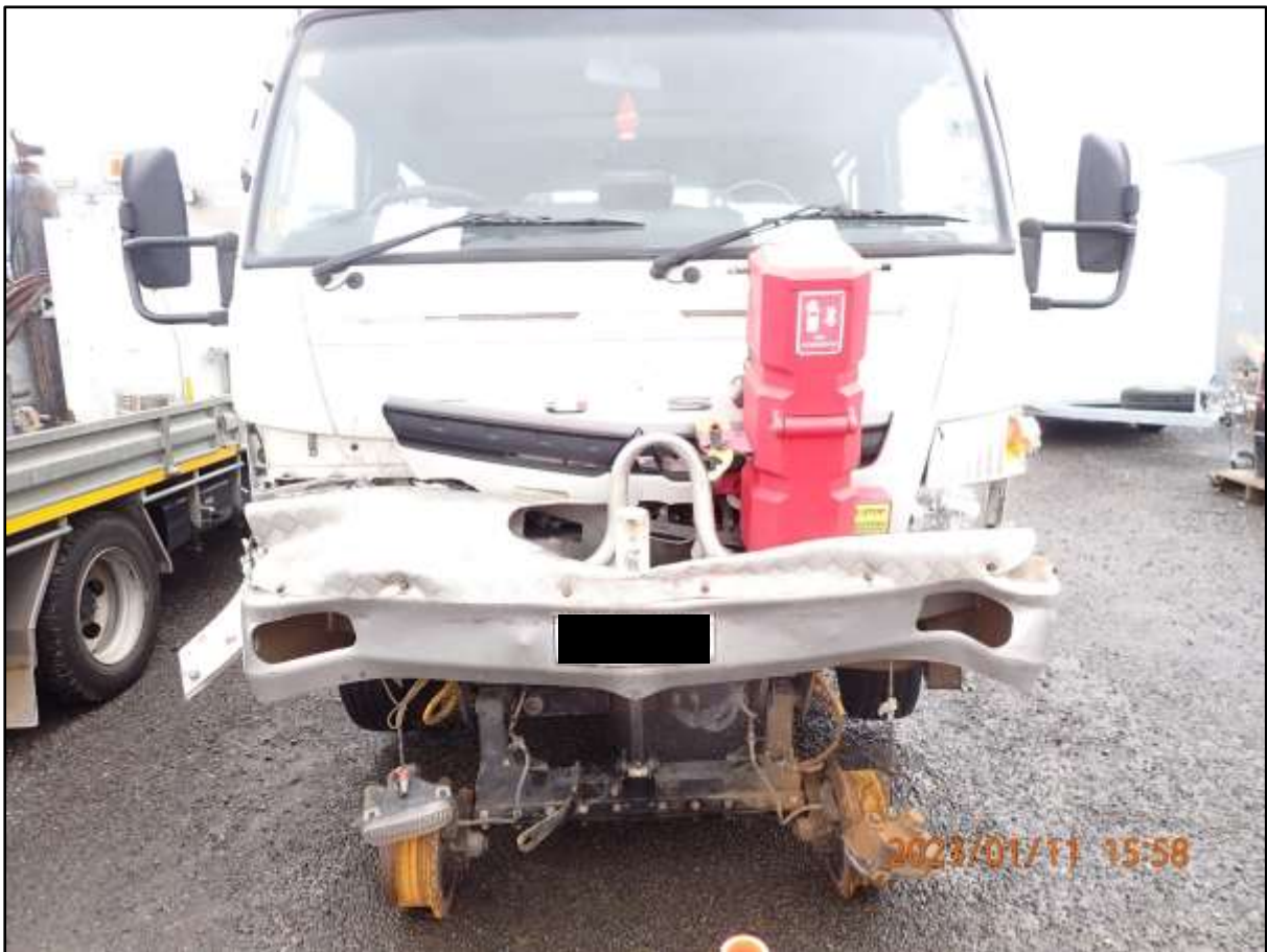
Figure 2: Hi-Rail vehicle 2 (HRV2) showing collision damage
