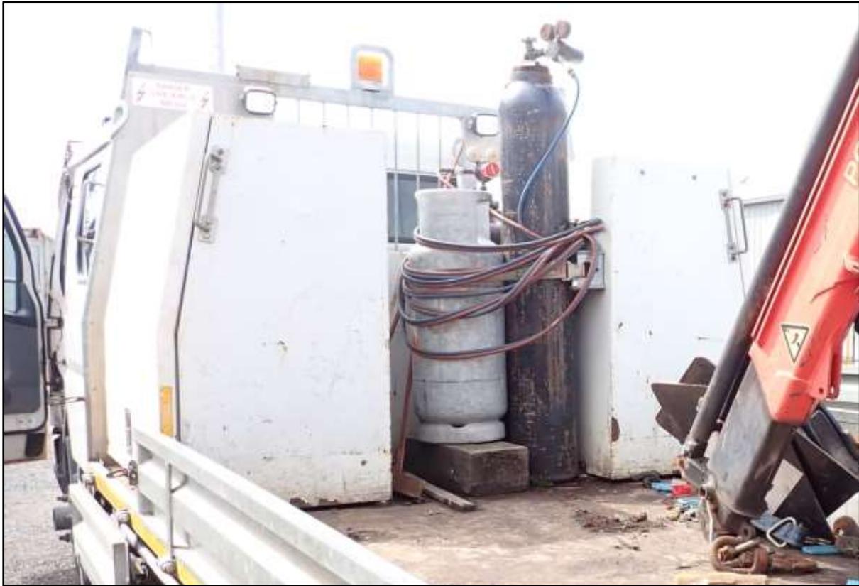
Figure 10: Gas bottles secured to metal cabinets on deck of HRV1
