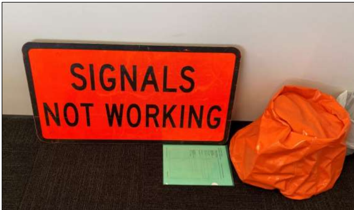
Figure 3: Sign and bag used when level crossing is disconnected
