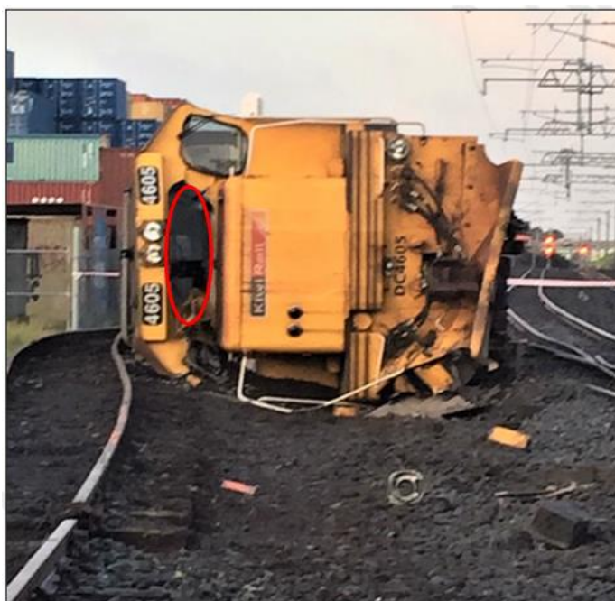
Figure 20: Locomotive following derailment, showing window through which crew exited.
