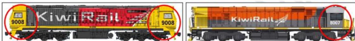
Figure 4: Dual-cab locomotive (left) and single-cab locomotive (right)
