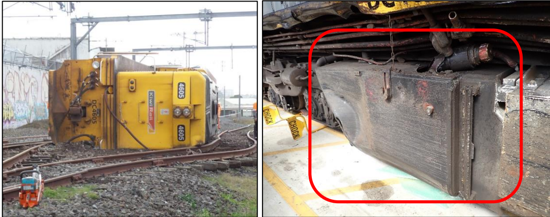
Figure 18: Position of locomotive following derailment (left) and ruptured fuel tank (right)
