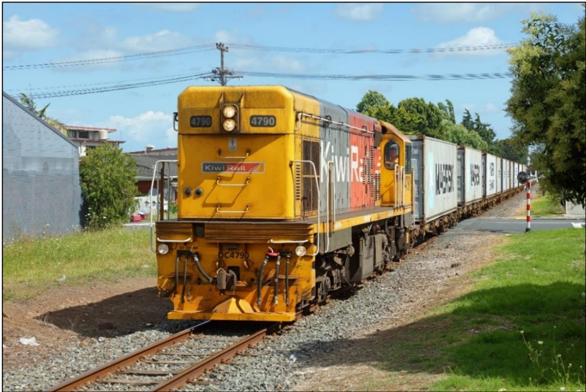
Figure 5: DC class locomotive operated in a long-hood leading configuration
