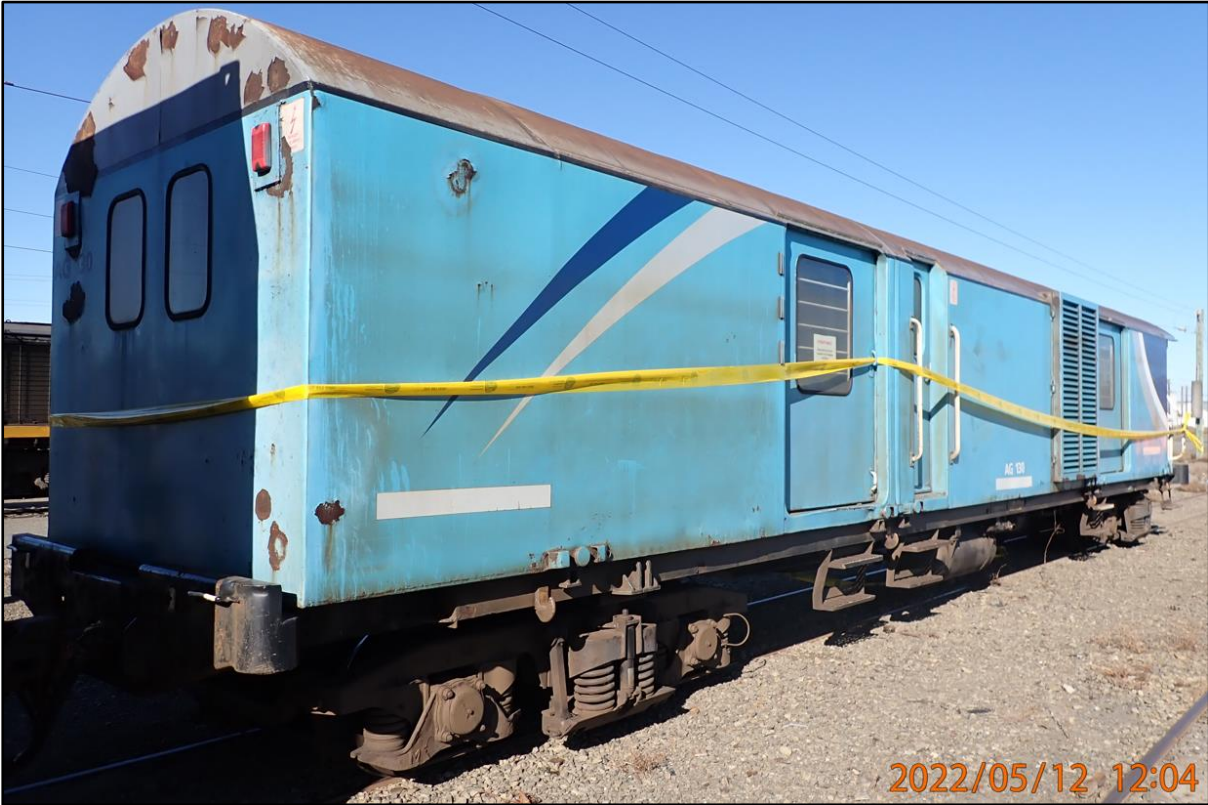
Figure 1: Auxiliary generator wagon 130
