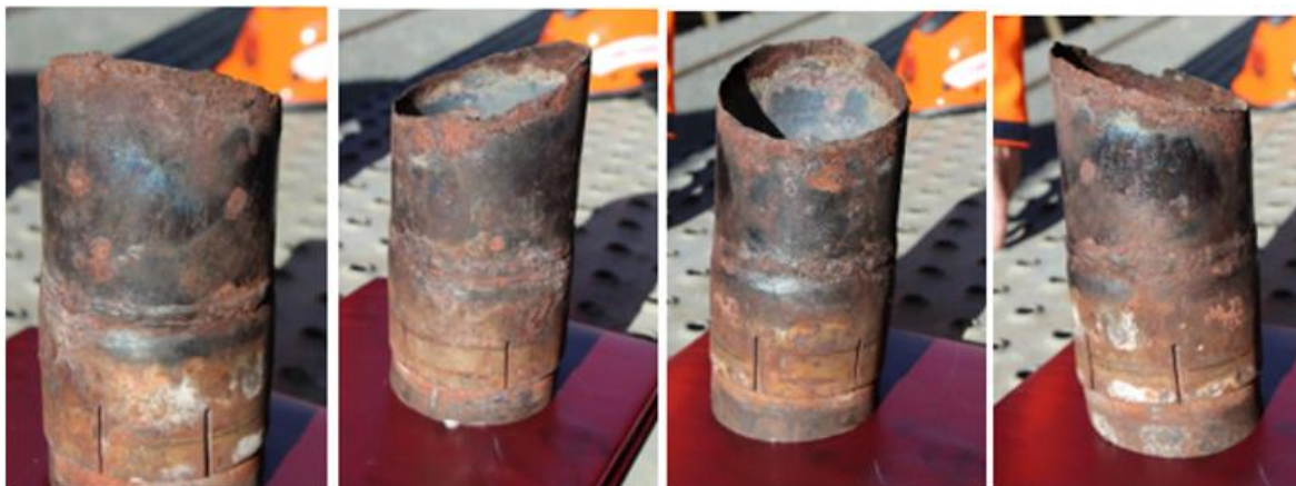
Figure 6: Exhaust tail pipe from AG130 after removal
