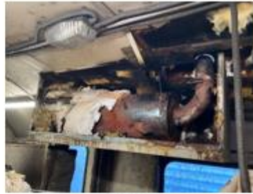
Photo 15. Exhaust silencer enclosure less insulation material AG130. IMG_2951.jpg
