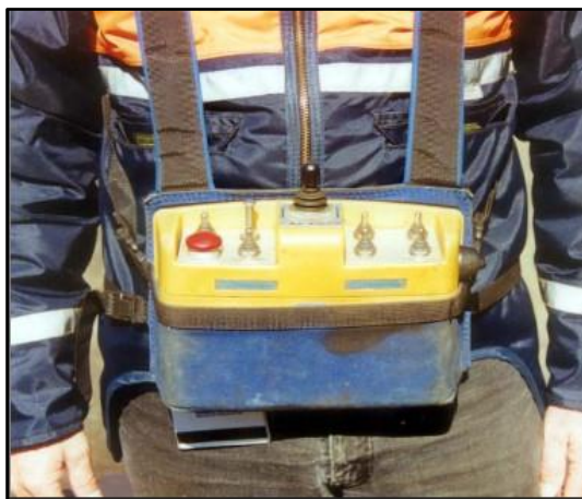
Figure 8: Remote-controlled pack worn in harness (Credit: KiwiRail)
