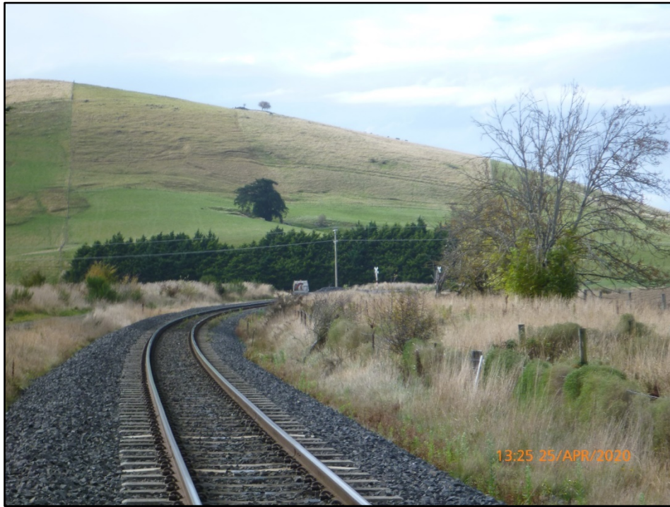
Figure 4: Sight line when the driver sounded the train horn (Credit: KiwiRail)
