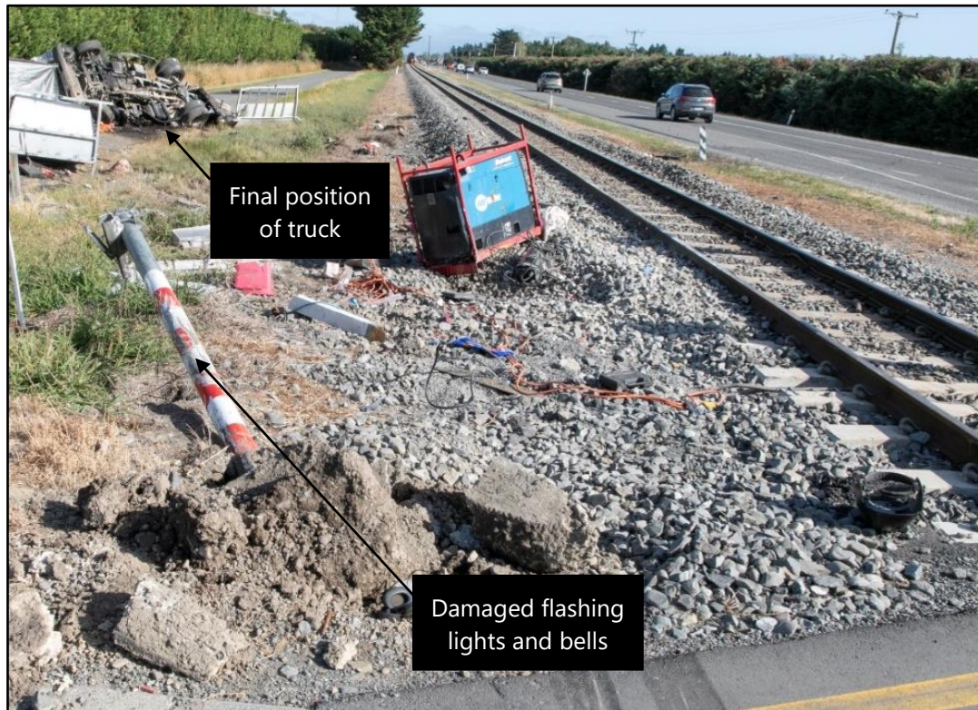
Figure 7: Damaged flashing lights and bells, and truck wreckage
