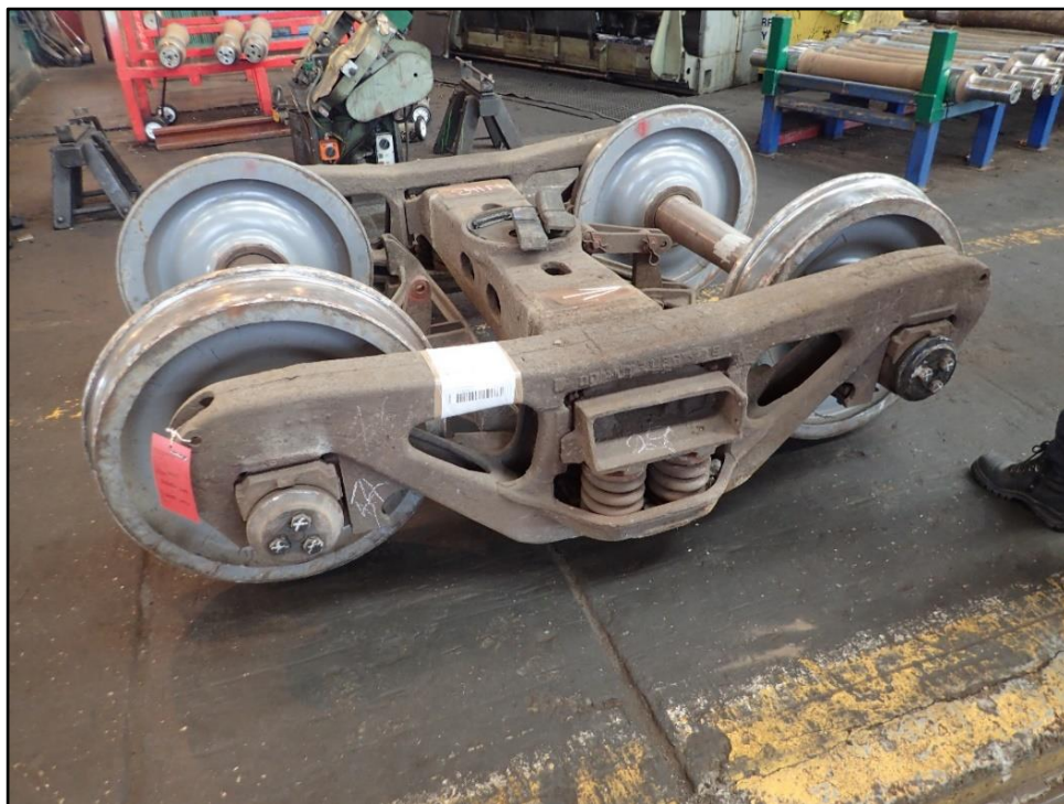
Figure 10: Leading bogie from UKN143 before examination
