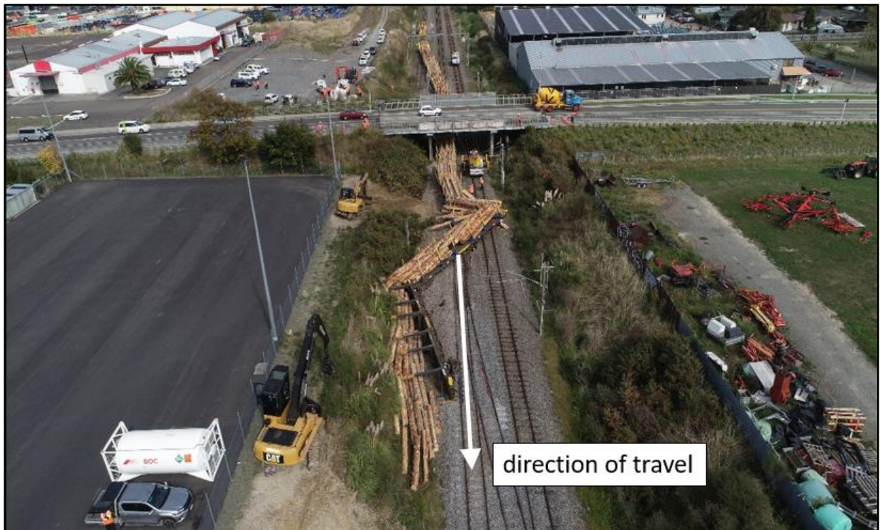
Figure 3: Derailed wagons (photograph provided by KiwiRail)
