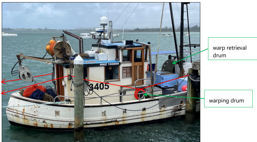
Figure 3: Boy Roel at the dock showing the typical trawl warp arrangement (red lines depict the trawl warp)
