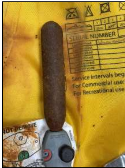
Figure 30: Corroded lifejacket cylinder
