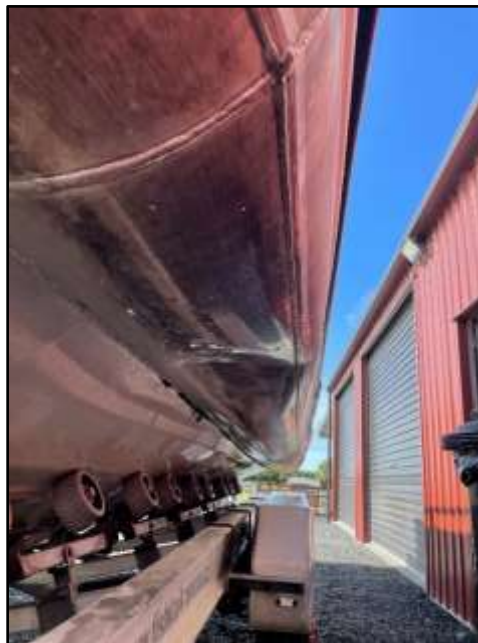
Figure 23: Indentation under port pontoon
