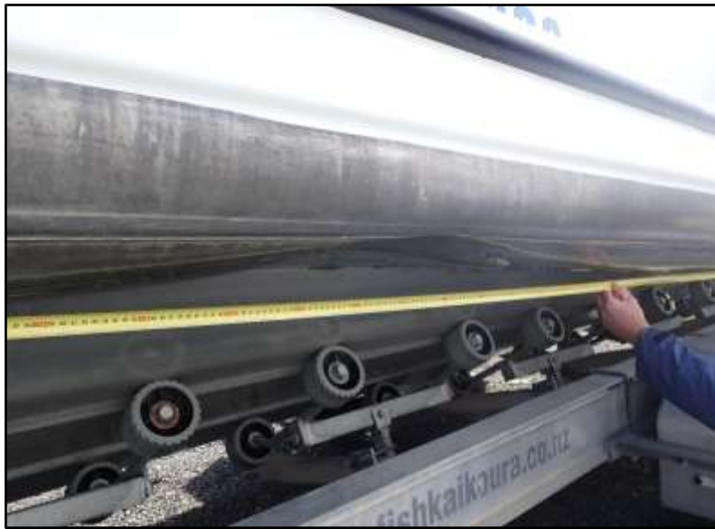
Figure 8: Indentation under port pontoon
