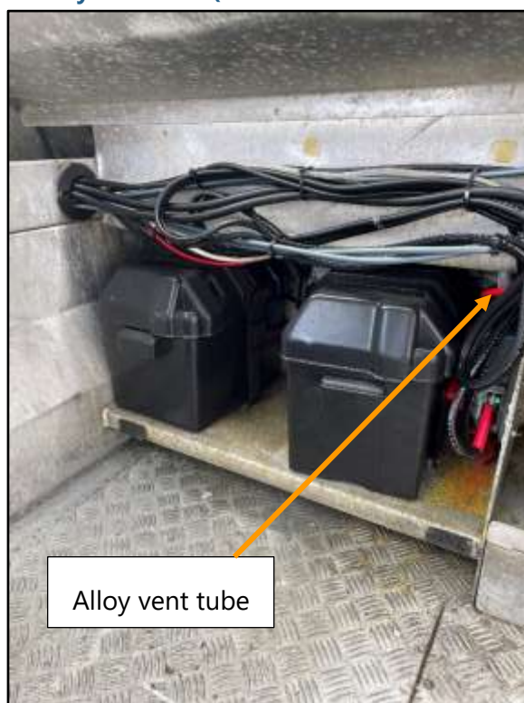
Figure 12: Location of alloy vent (after accident)
