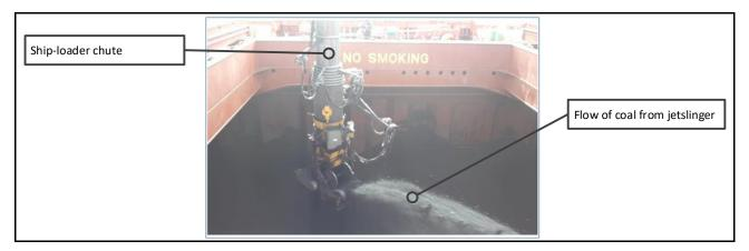
Figure 17: Jetslinger in operation, loading coal onto a different vessel
