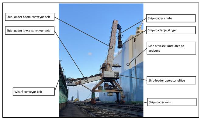
Figure 16: LPC ship-loader in its stowed position next to a car carrier vessel
