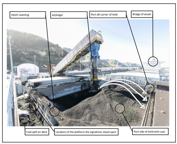
Figure 18: Number one hold after the accident, showing the ship-loader and jetslinger<sup>95</sup> (Credit: Maritime New Zealand)
