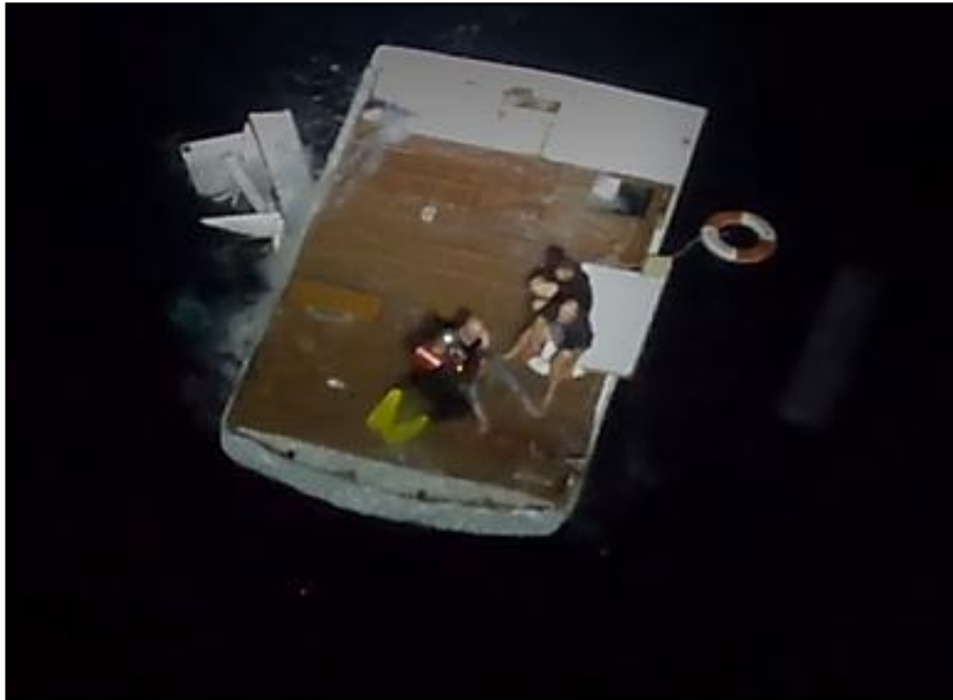
Figure 18: The inverted flybridge with a rescue swimmer and three survivors sitting atop what had been the ceiling of the main saloon and the floor of the flybridge
