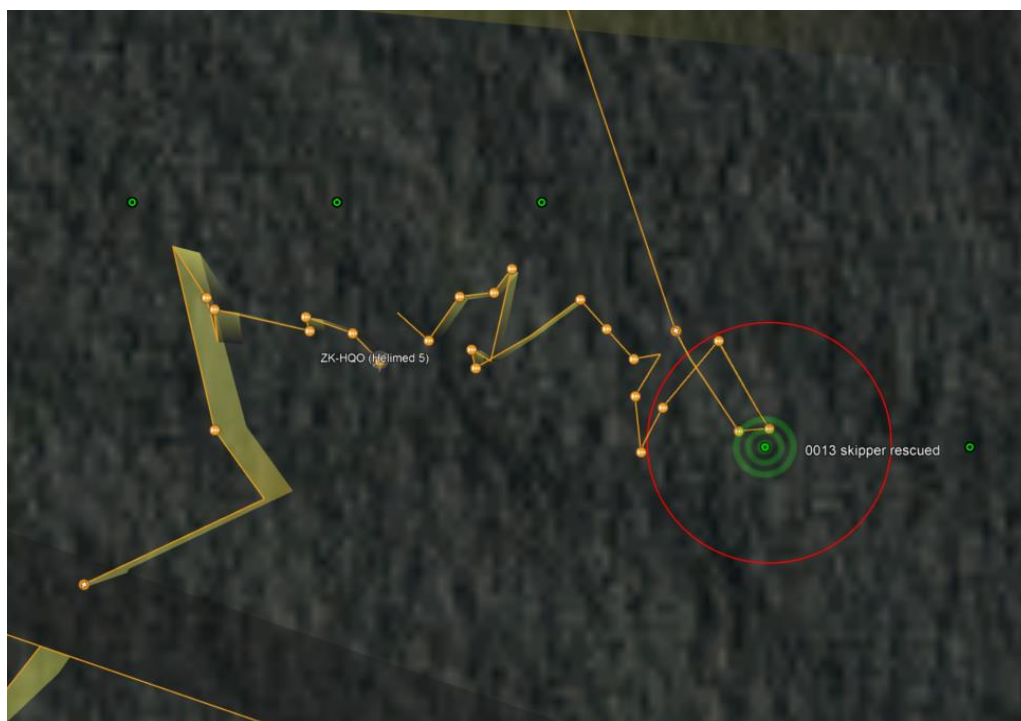
Figure 33: Flight data showing helicopter hovering over EPIRB encoded position (green dots)
