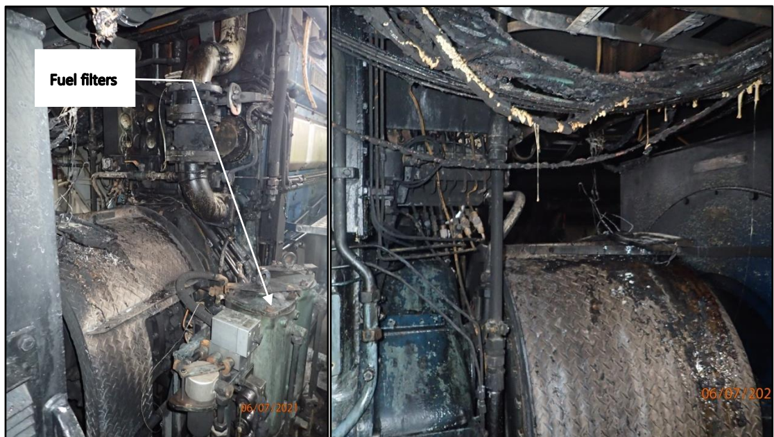
Figure 7: Photographs of general heat and smoke damage around the seat of the fire (left) and heat damage to electrical cables and fittings (right)
