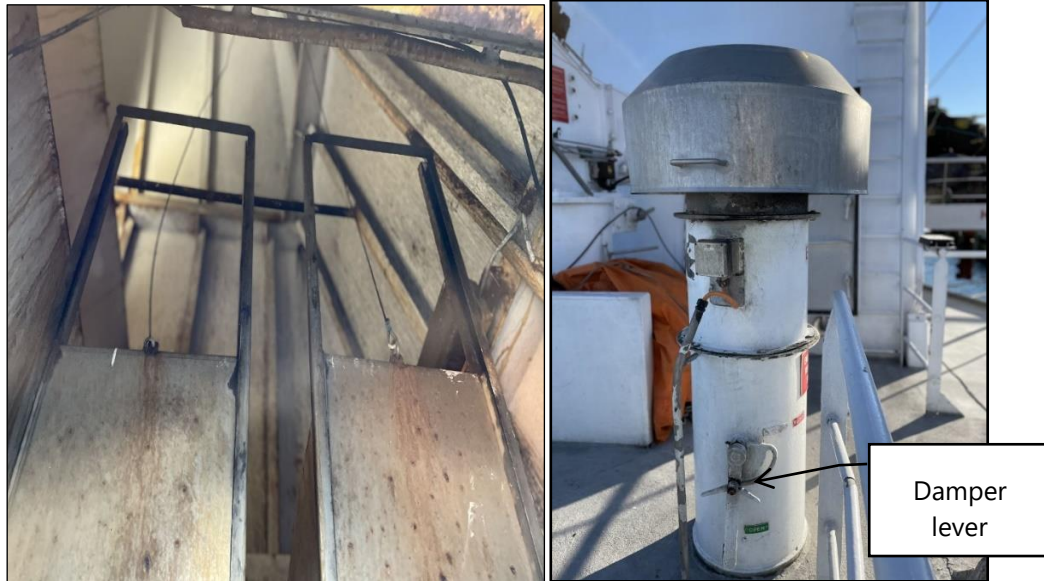
Figure 4: Photographs showing sliding dampers that when released drop down in their guides to seal off the opening (left) and No. 2 extraction fan with the lever for opening and closing the butterfly damper on the trunking (right)
