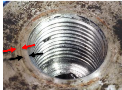
Figure 5: End of the new accumulator showing the condition of thread and minor marks from the rubber seal (black arrows) and steel outer (red arrows) of the connector.
