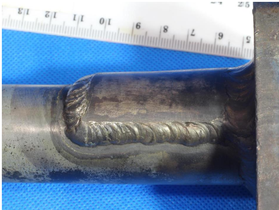
Figure 10: Repair weld and doubler plate.
