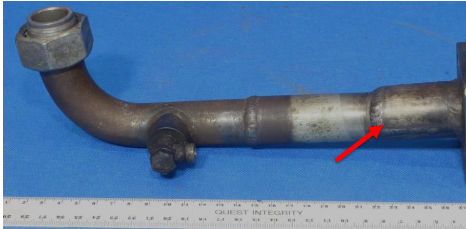
Figure 9: Pipe fitting. Showing the patch repair (doubler plate) over the leak (arrowed).
