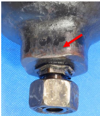
Figure 2: Old accumulator showing damage paint in area arrowed.
