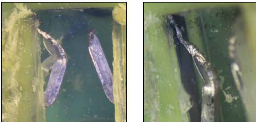
Figure 10: Example of the condition of a similar fuse deliberately failed through electrical overload
