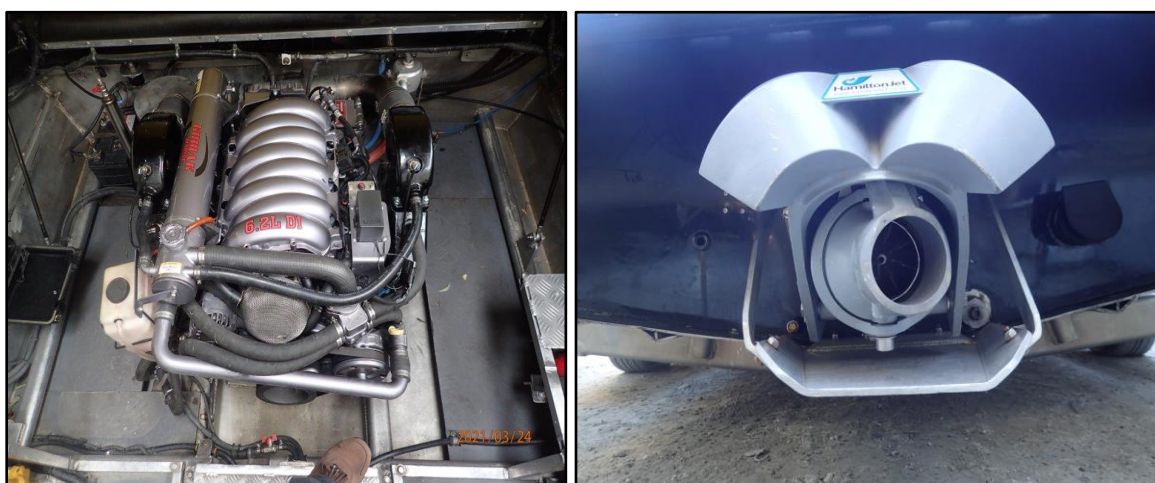
Figure 4: Left – single 6.2 litre DI V8 Kodiak (Chevrolet) engine. Right – Hamilton Jet type 212 jet unit
