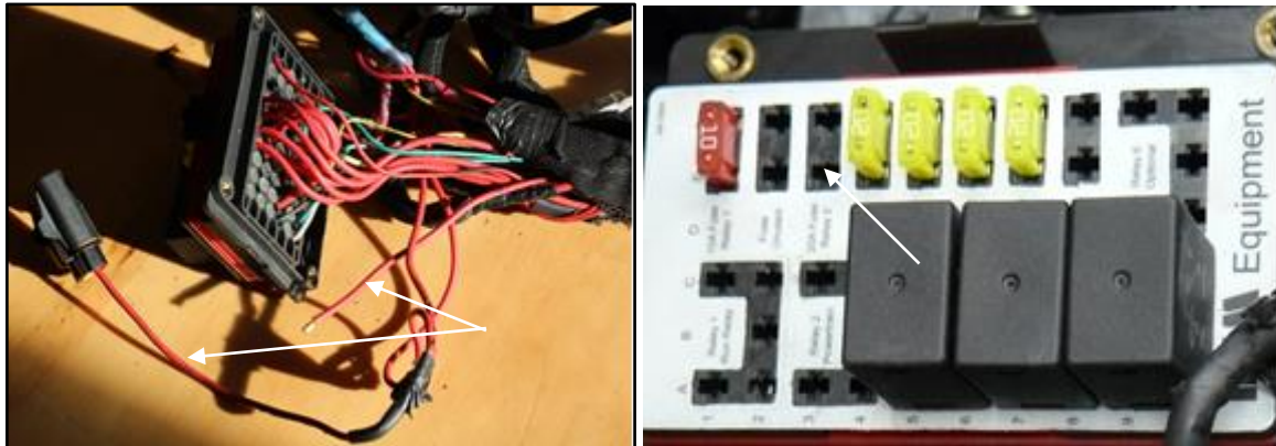
Figure 11: Left – wiring loom at the rear of the fuse box from KJet 8 showing the two wires that had been attached to the failed fuse. Right – fuse box where the failed fuse had been located
