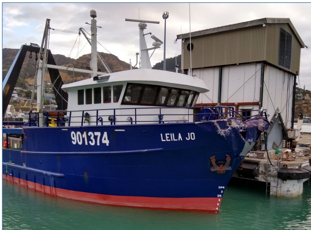
Figure 7: Post-accident photograph of damage to Leila Jo (Credit: Archie Laird)
