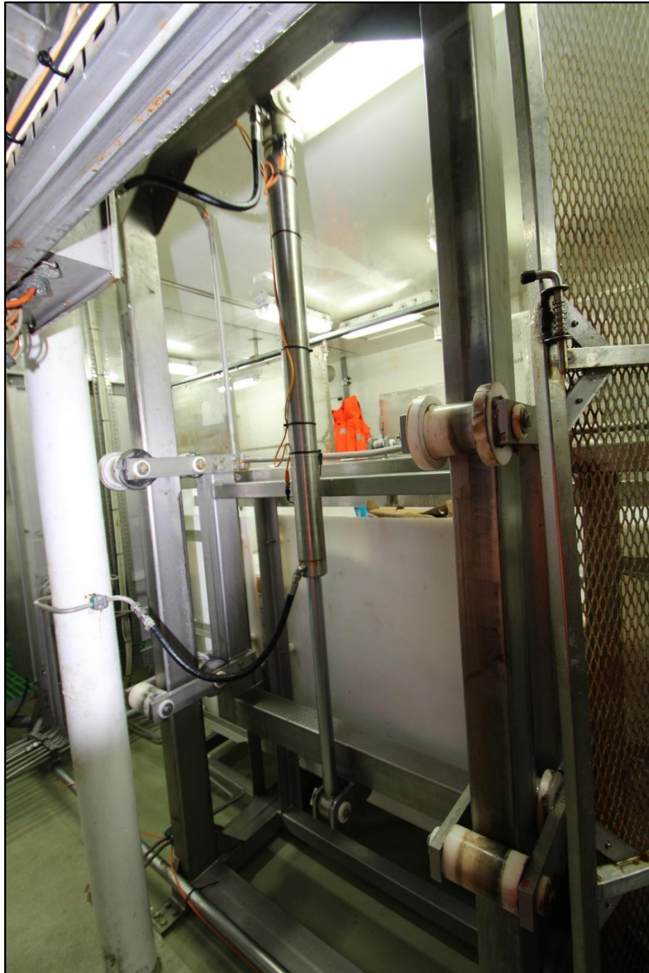
Figure 7: Hydraulic ram at the back of the accumulator, which moves the floor up and down (credit: Maritime New Zealand)
