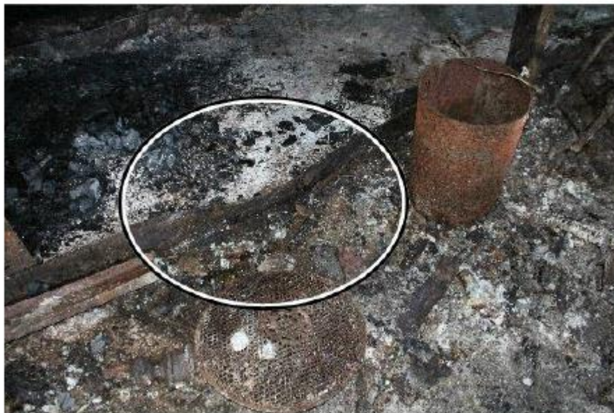
Photo 12: The circle shows the warped steel plate.
