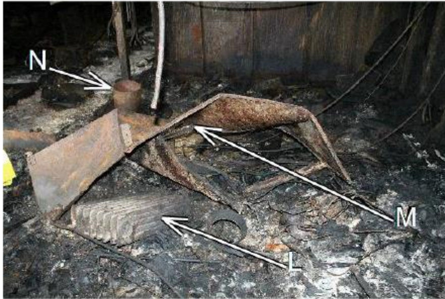
Photo 11: Shows the first engineer's cabin looking to the rear of it. 'M' identifies the fridge. Note the way it has collapsed. 'L' identifies the oil column heater. 'N' identifies the rubbish bin.
