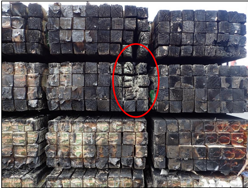
Figure 9 Timber packet showing origin of fire
