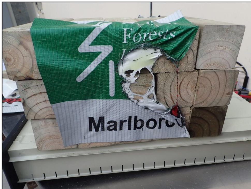
Figure 7 Plastic wrapping after two minutes, 20 seconds of exposure to the ship's lamp
