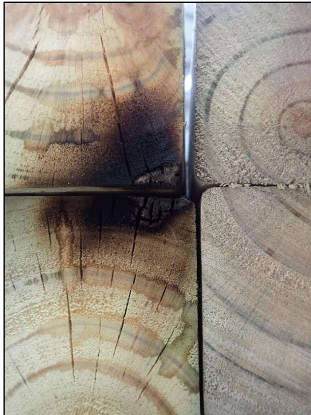
Figure 5 Photograph taken after three minutes' exposure to the lamp
