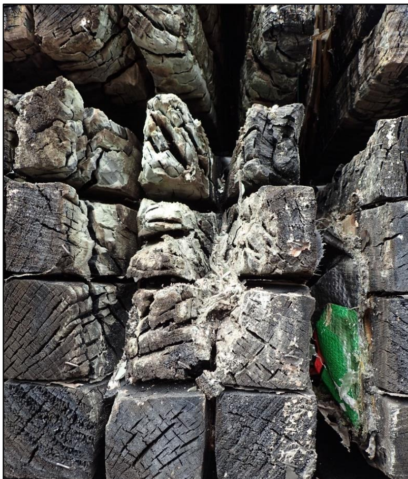
Figure 10 Charred timber at origin of fire
