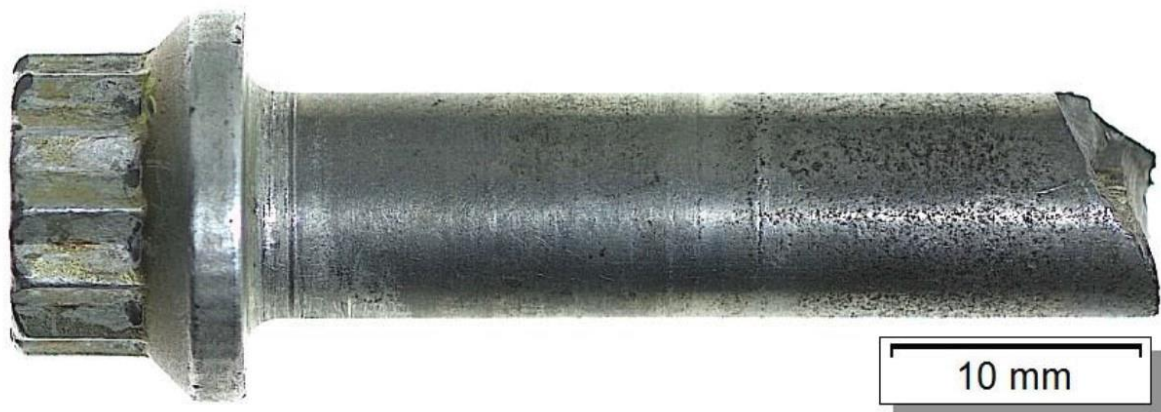
Figure 4: Broken fastening bolt with a conspicuously snarling surface in the fracture area.
