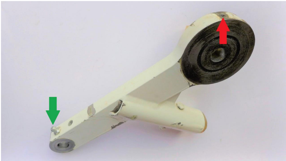
Figure 5: Upper arm of the torque link with an intact lubricating nipple (left green arrow) and the broken and file-processed lubricating nipple of the affected joint (right red arrow).
