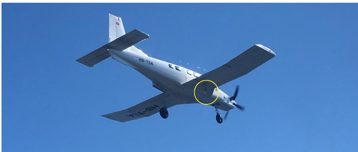
Figure 1: The HB-TSA with the landing gear stump without a wheel (yellow circle) after dropping the parachutists, taken from a Swiss Air Force aircraft.
