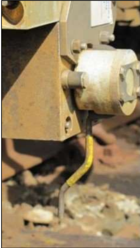
Figure 3: Train stop trip lever fitted to Transdev passenger trains
