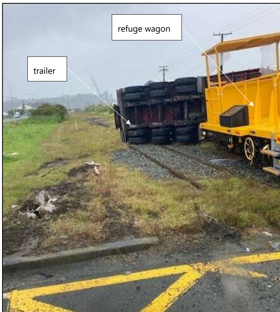
Figure 6: Truck trailer and refuge wagon after the collision
