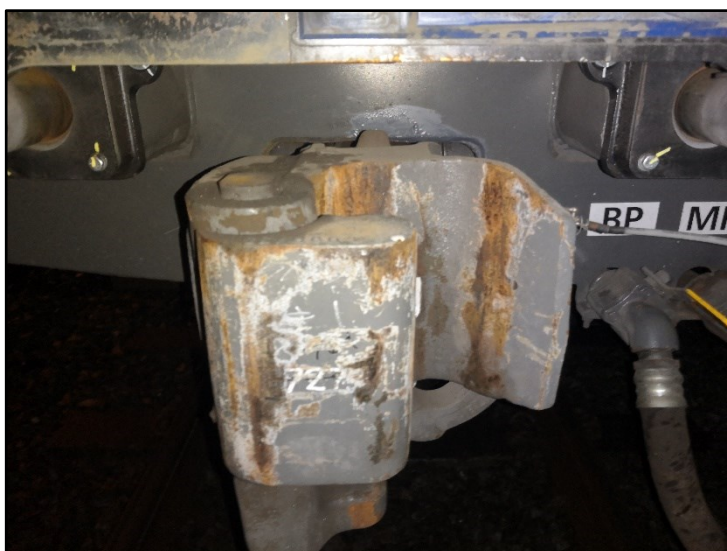
Figure 9: Third carriage – front coupler in closed position after second parting
