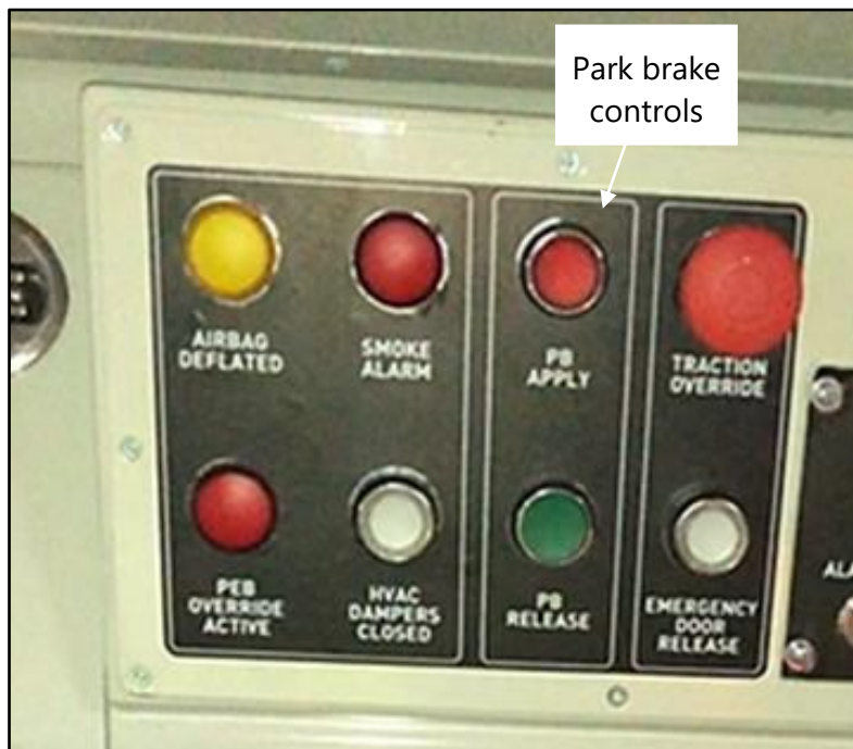
Figure 19: Overhead control panel for DFB class locomotive with running capability
