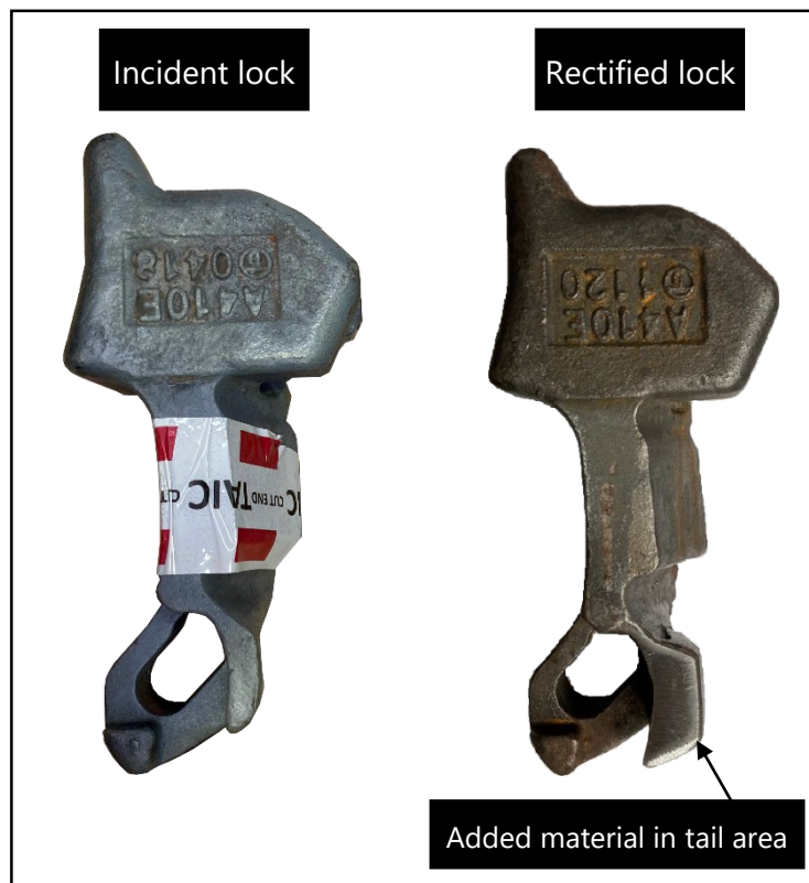
Figure 24: Incident lock and lock modified to correct lacking material in tail area
