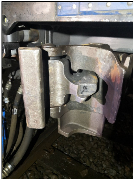
Figure 8: Second carriage – the rear coupler in open position after second parting
