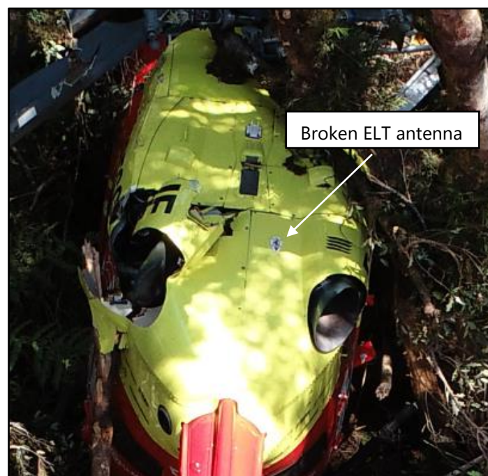
Figure 15: broken ELT antenna after the accident sequence
