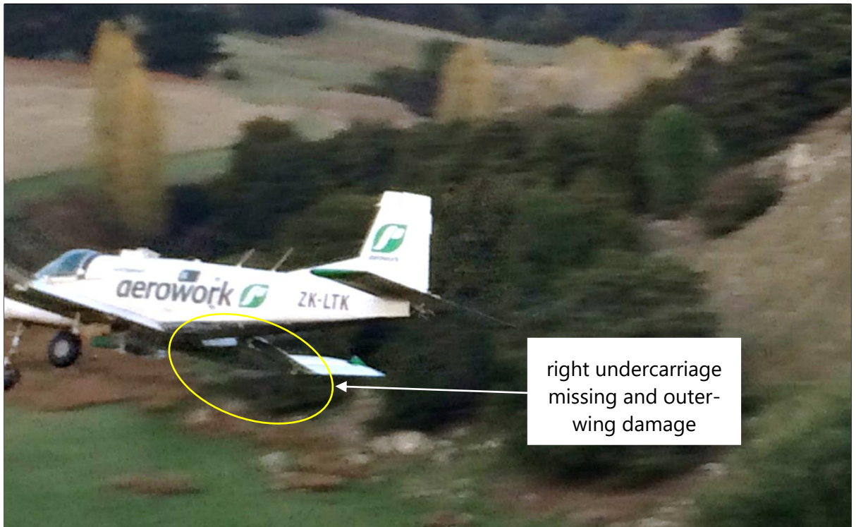
Figure 7: Undercarriage missing and right-hand-wing damage (Credit: G Saunders)
