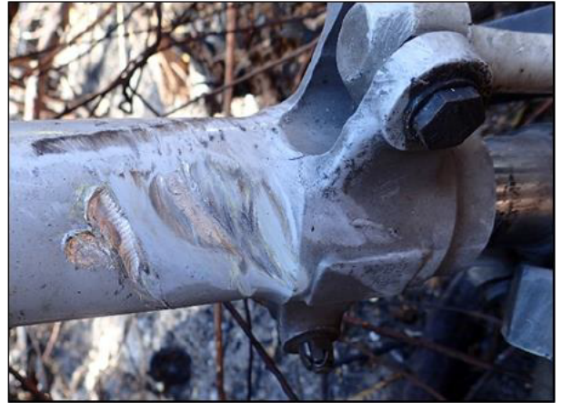
Figure 7: Impact damage to the pitch control mechanism
