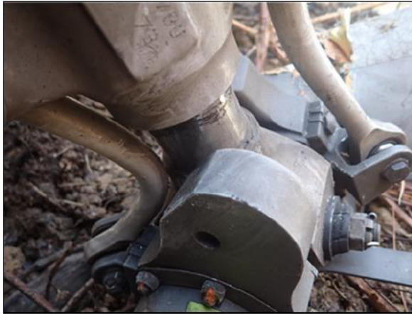
Figure 6: Pitch control links bent inward
