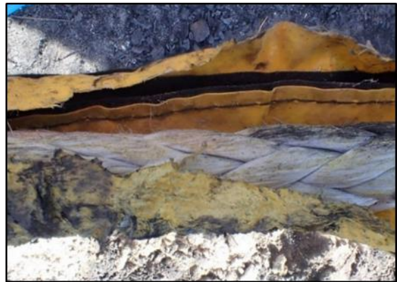
Figure 13: Damage to the lifting line sheathing material
