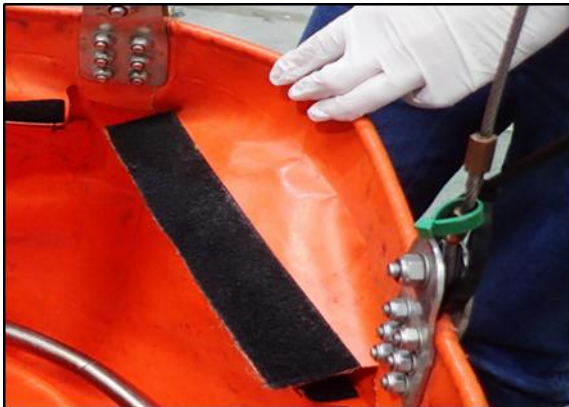
Figure 12: Bucket in collapsed state in situ at the accident site
