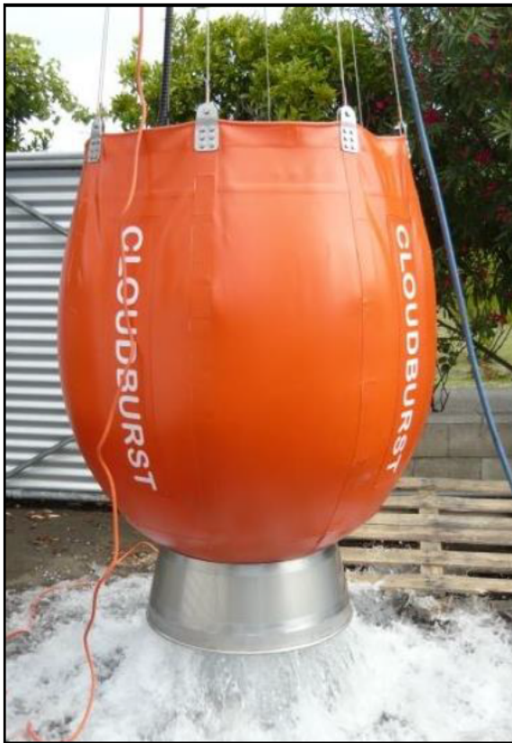
Figure 16: Cloudburst 1000 bucket filled during testing (credit: IMS New Zealand)
