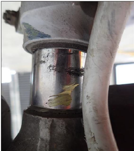
Figure 8: Yellow material transfer on to tail rotor assembly
