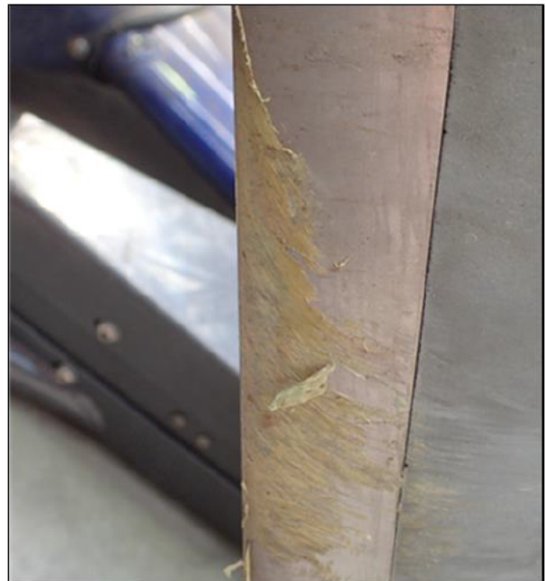
Figure 9: Yellow material transfer on to tail rotor blade
