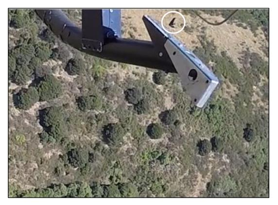
Figure 9 The vertical stabiliser falling to the ground (cropped image)
