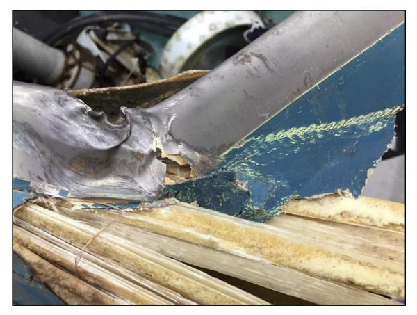
Figure 3 Damage to the leading edge of one of the tail rotor blades
