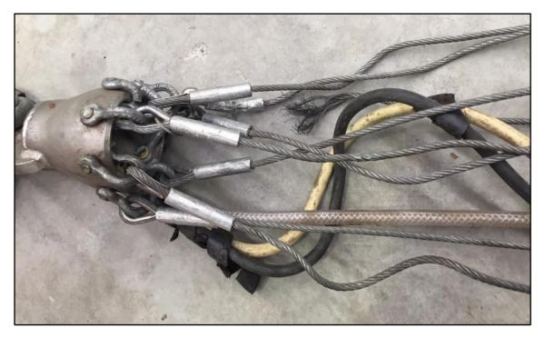
Figure 4 The monsoon bucket cable cluster with broken shackles and damaged cables
