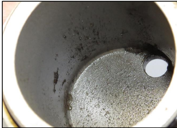
Figure 4 Fuel filter housing showing sludge residue
