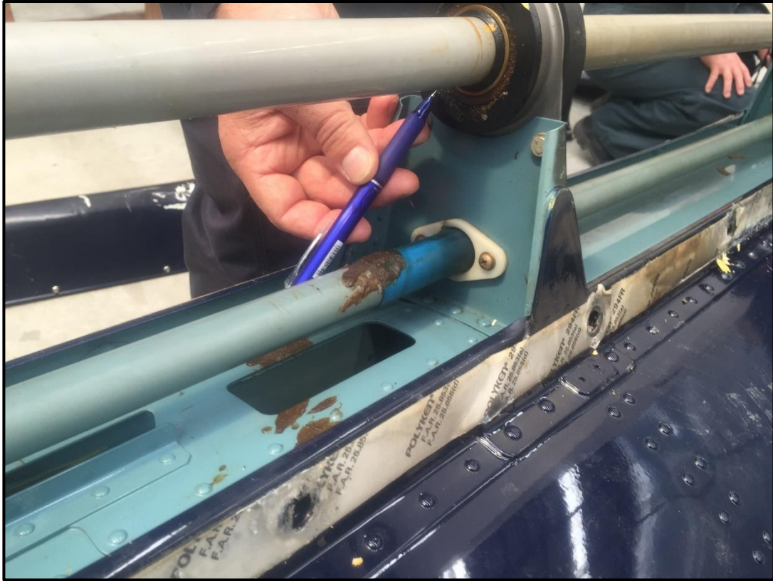
Figure 10 Grease throw on tail rotor drive shaft
