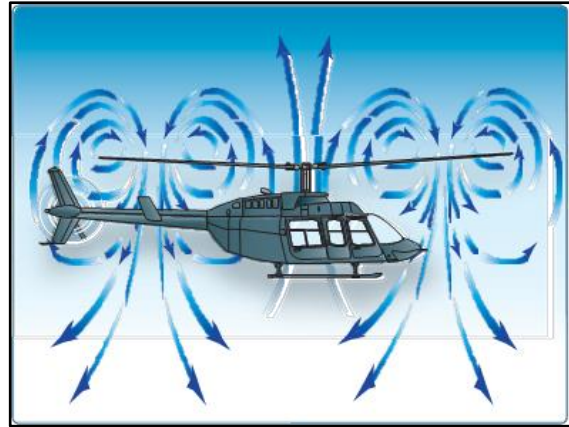
Figure 12 Vortex ring state (Courtesy of Federal Aviation Administration)
