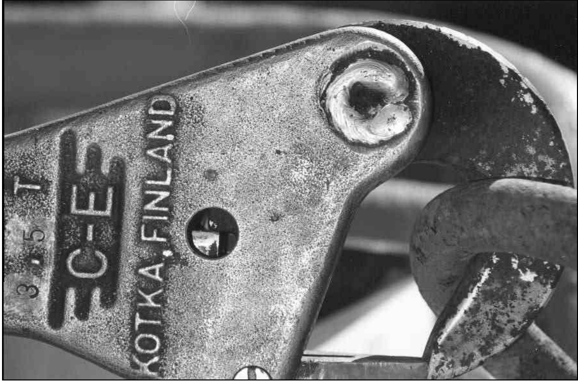
Figure 6 View through the aperture of the locking pin partially engaged with the hook locking face (by about 3 to 4 mm)
