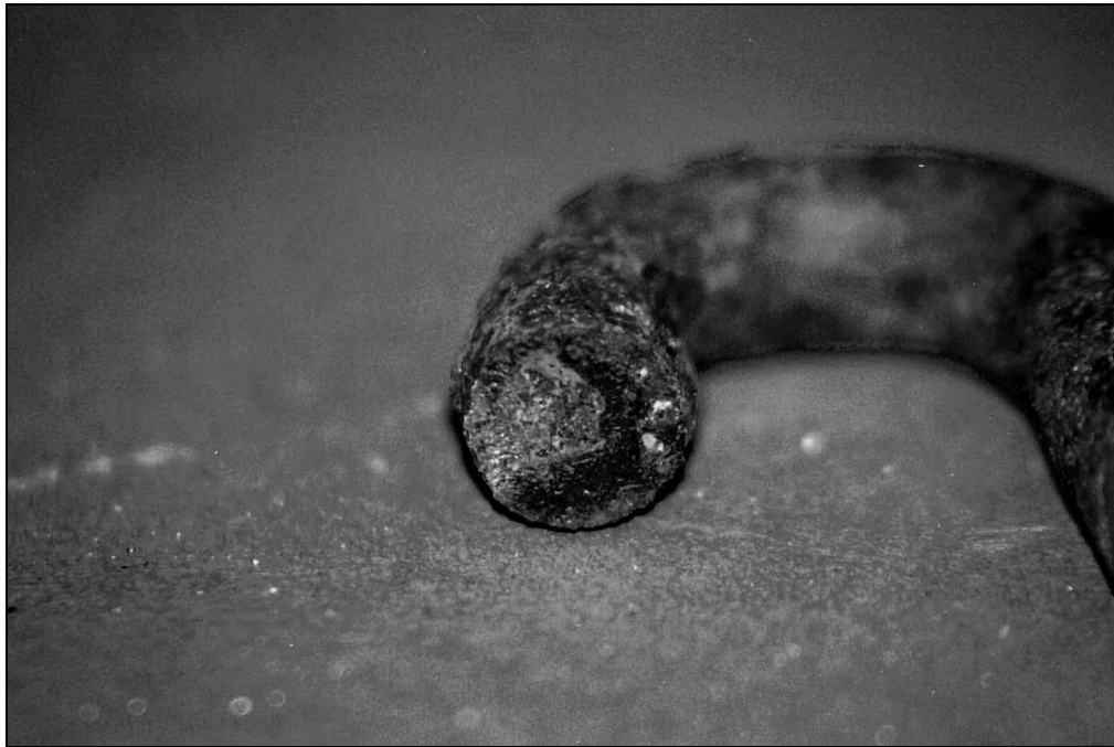
Figure 8 Brittle fracture of failed link from preventer chain
