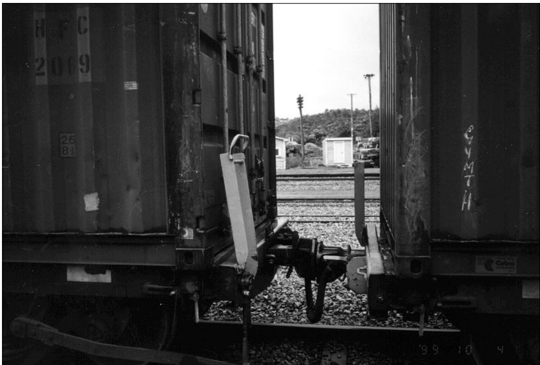
Figure 5 Example of a handgrip bent inwards
