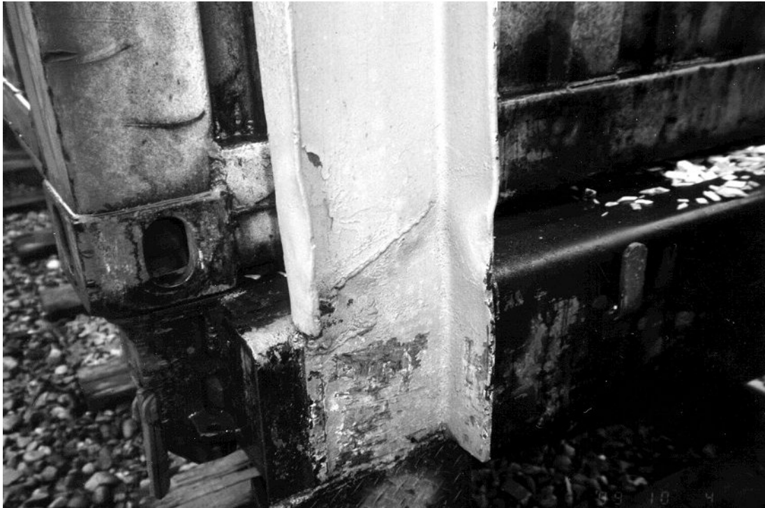
Figure 8 Example of a handgrip which had been repair welded
