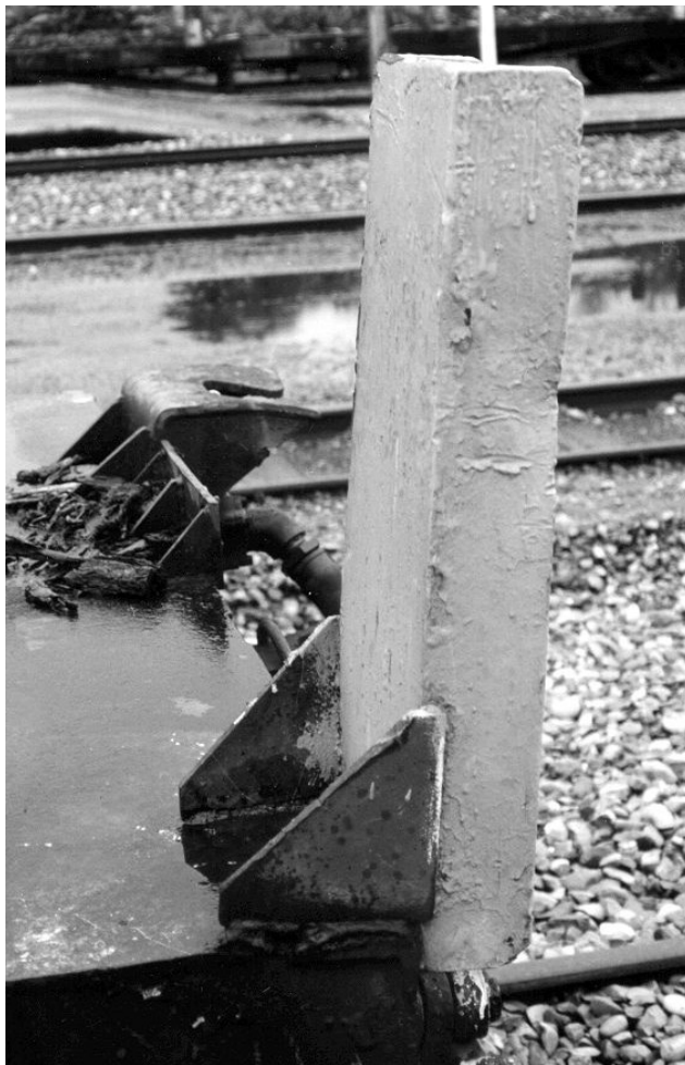
Figure 6 Example of a handgrip bent outwards
