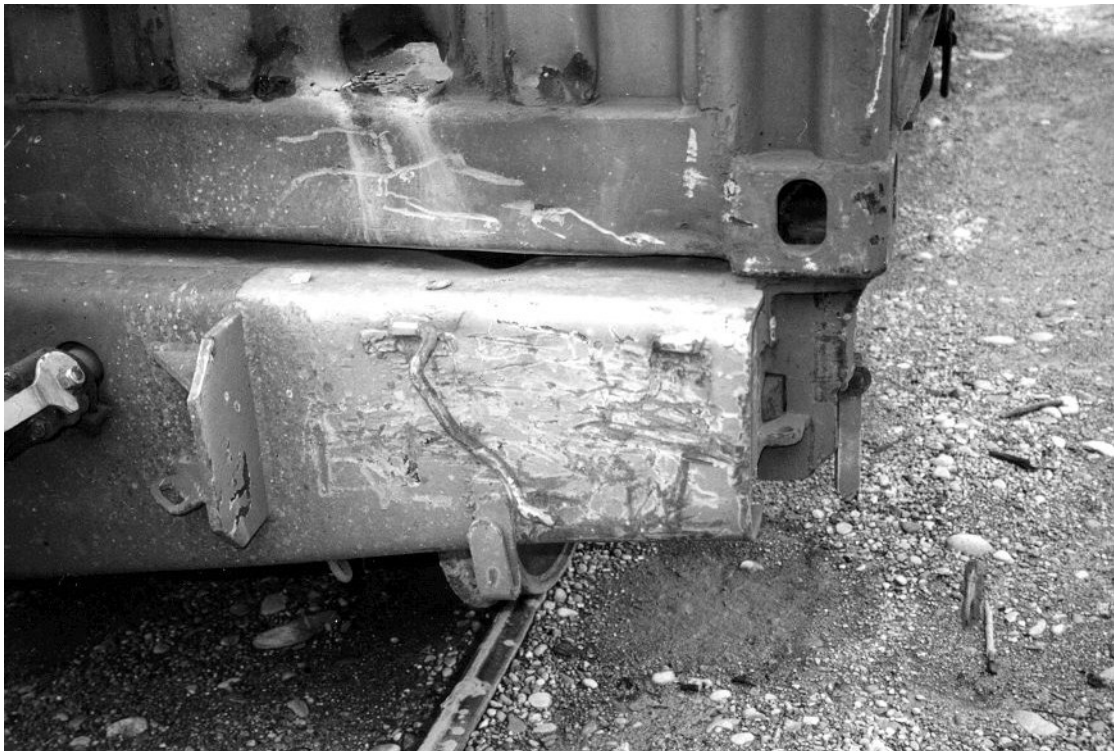
Figure 10 Typical damage to a coupling handgrip, headstock and container
