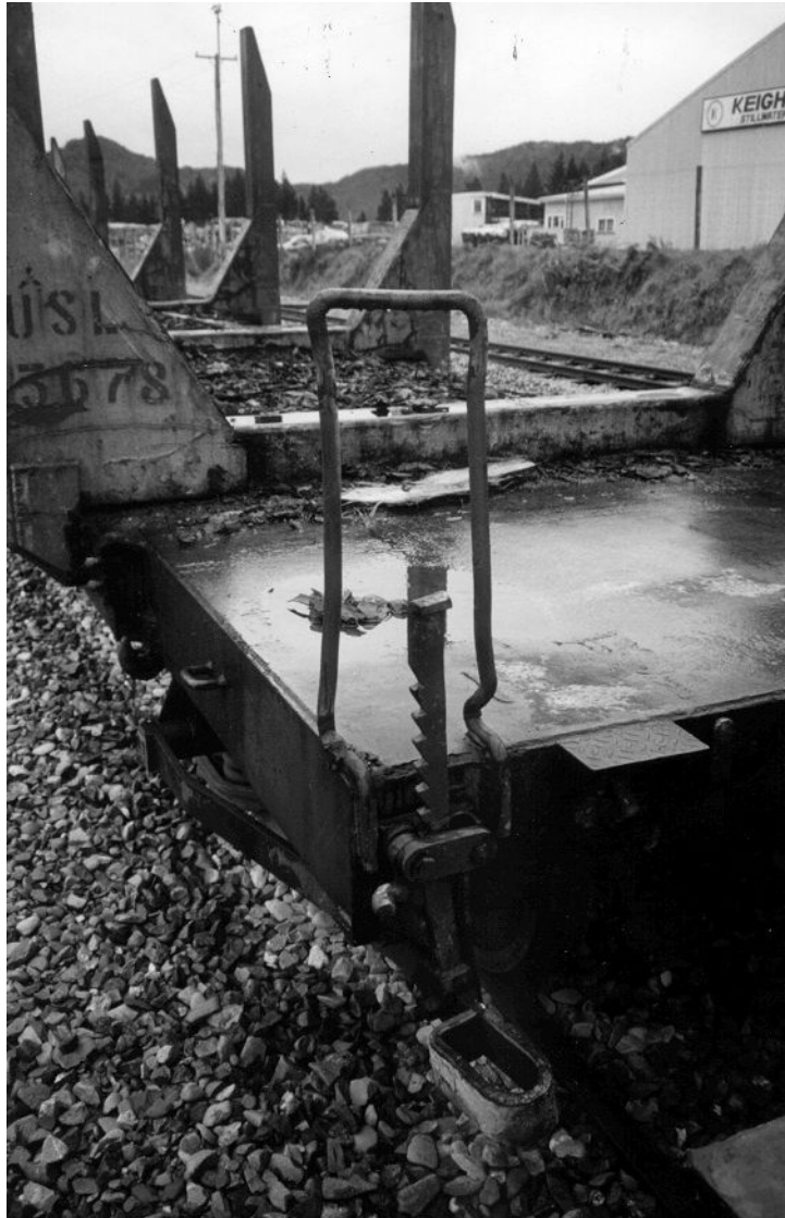
Figure 9 The new hoop style handgrip in service
