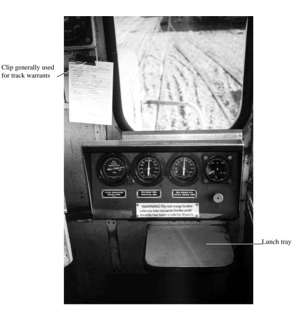
Figure 2 The position of the track warrant clip in a DBR class locomotive cab (similar profile and configuration to a DC class locomotive cab)
