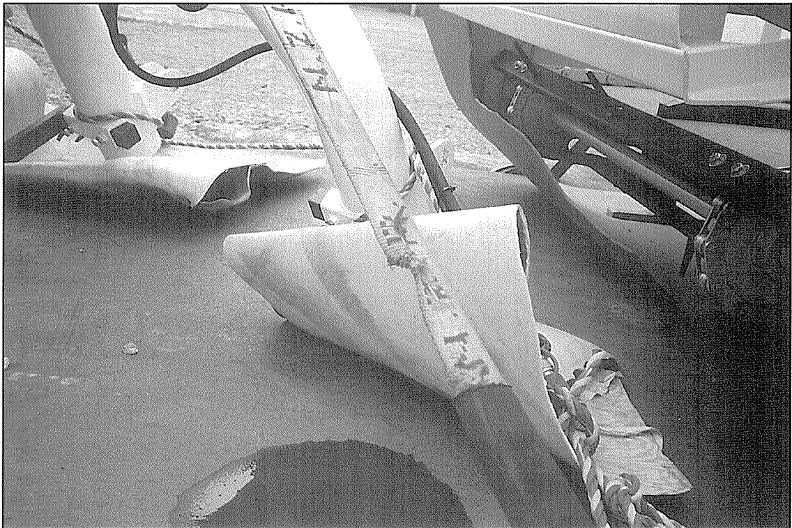
Figure 3 Partially severed strop used on wagon US3985
