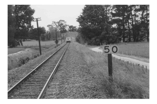
Figure 6 Curve Warning Board at 129.828 km
