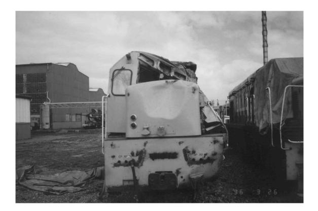
**Figure 7** Damage to cab of DX 5310
