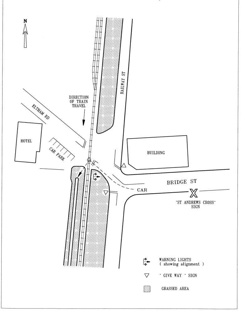
lights. One set of warning lights was aligned to face westbound traffic on Bridge Street, and this set was visible from within 190 m of the crossing. The crossing itself was not directly visible to the driver on this approach until he
