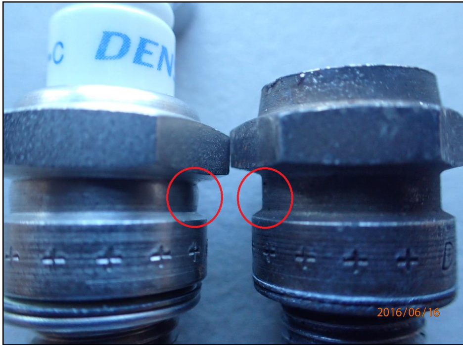
Figure 8 Difference in length compared with a new plug (on left), and comparison of 'bulge' (circled)
