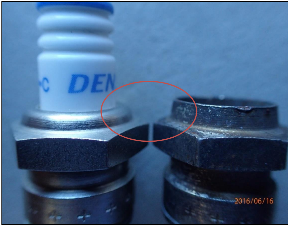
Figure 7 Number 4 spark plug shell (on right), flange not formed
