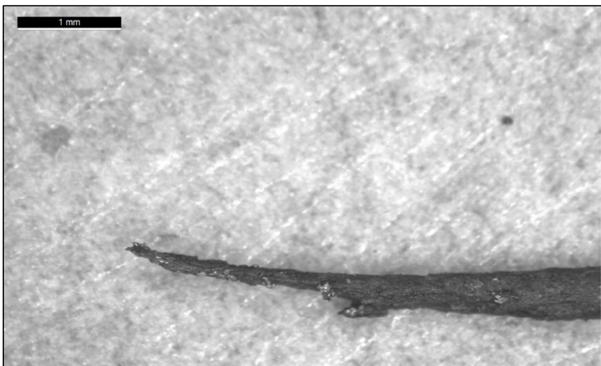
Figure 7. A single severely corroded wire extracted from the failure zone
