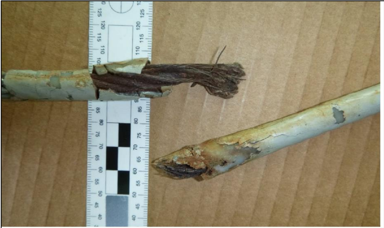
Figure 1. Failed ends of the rope upon receipt
