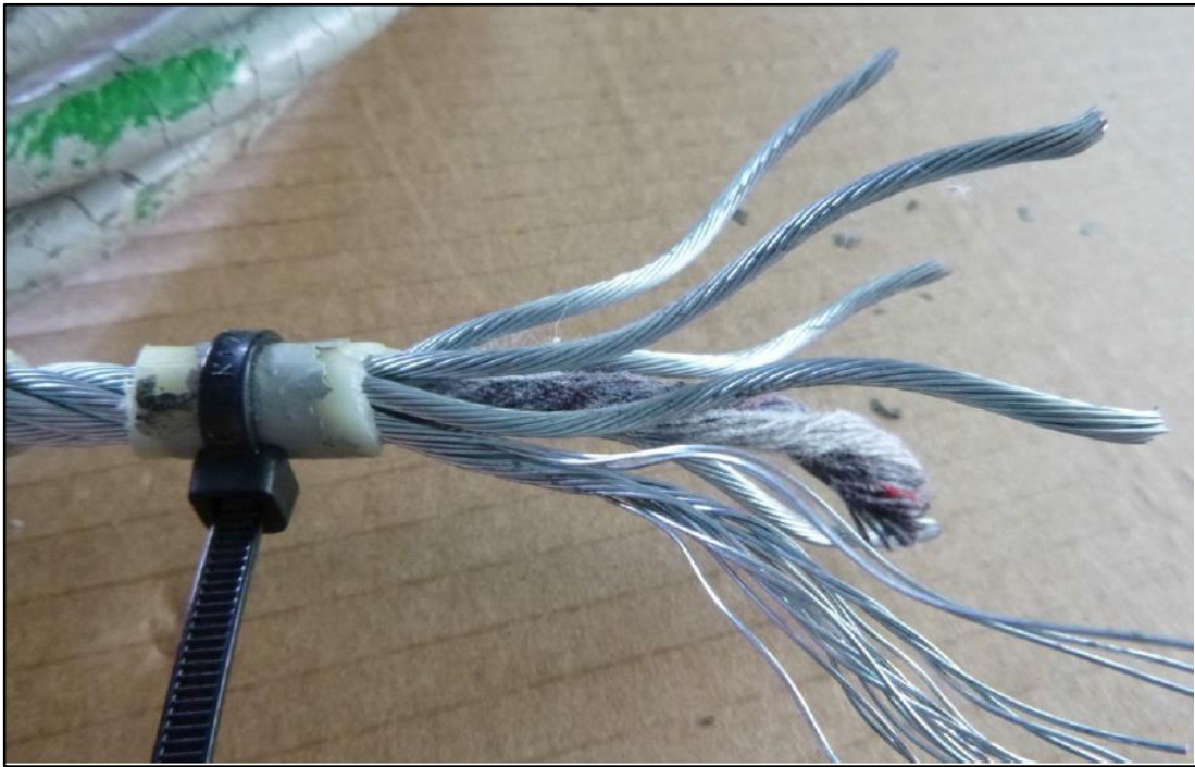
Figure 5. Uncorroded condition approximately 900 mm from the point of failure
