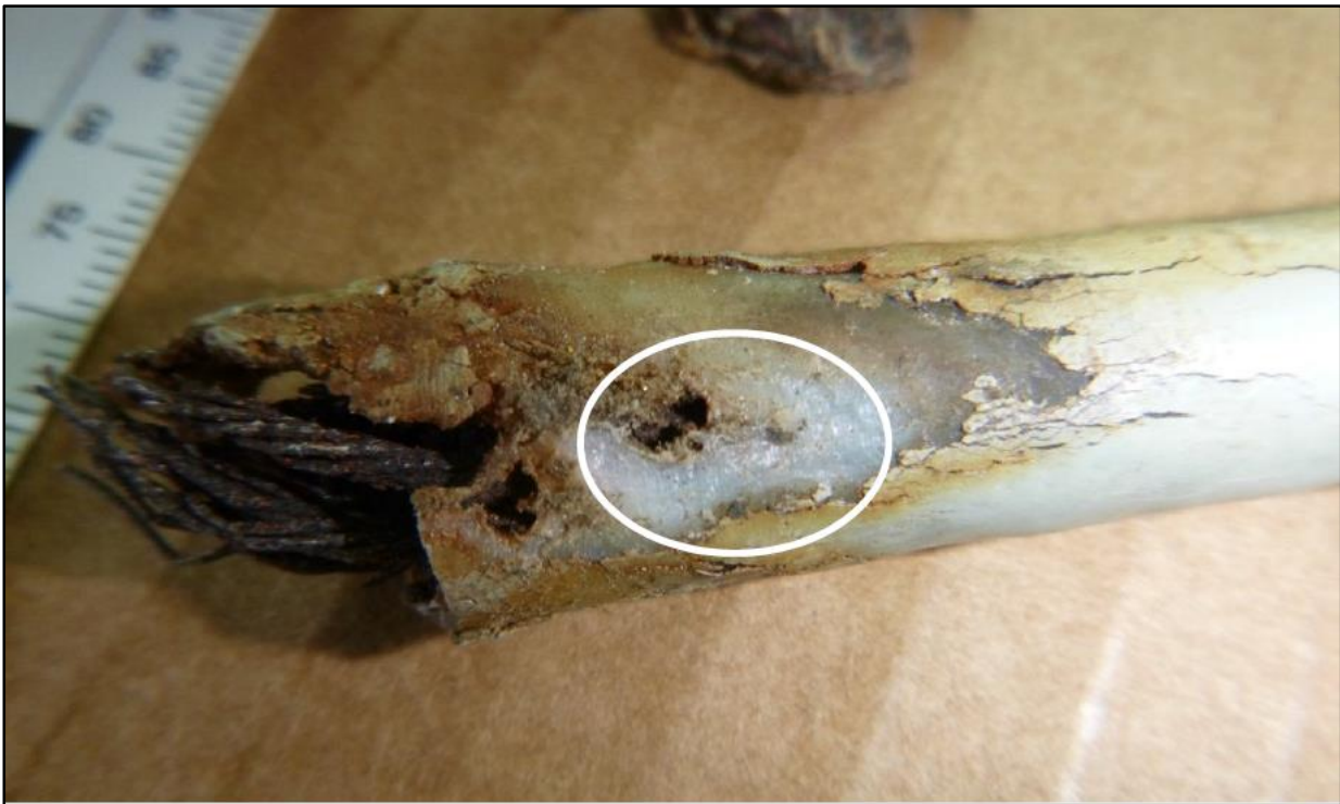
Figure 2. Local degradation of outer sheathing and fresh abrasions (circled).
