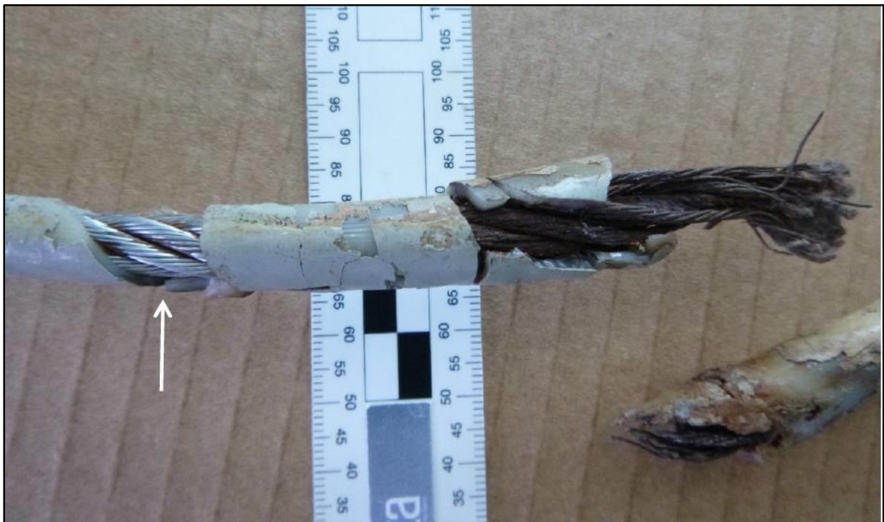
Figure 4. Relatively uncorroded wires present close to the failure (indicated by arrow)
