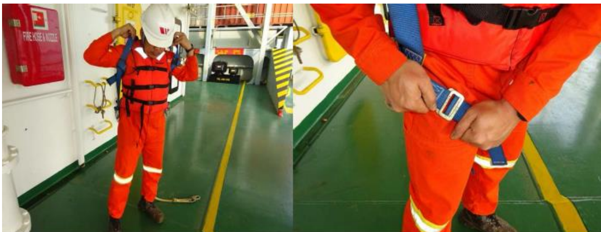
Wear the safety harness and ensure that the thigh straps are properly tightened.
