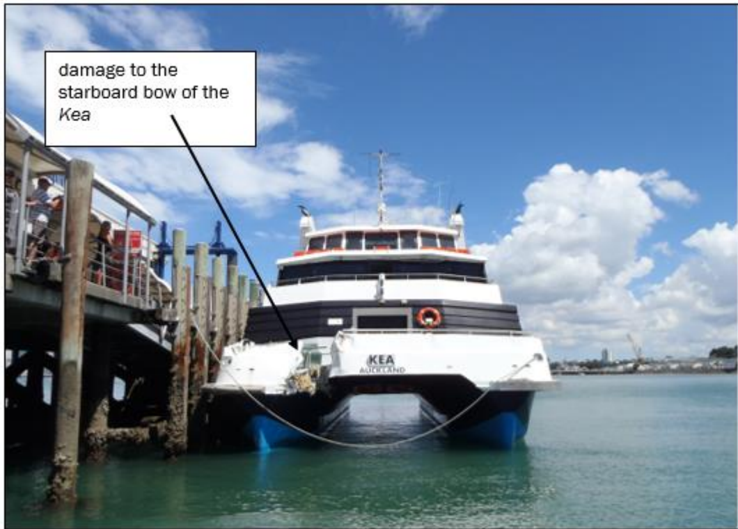
Figure 6 Impact damage to the Kea's starboard bow area
