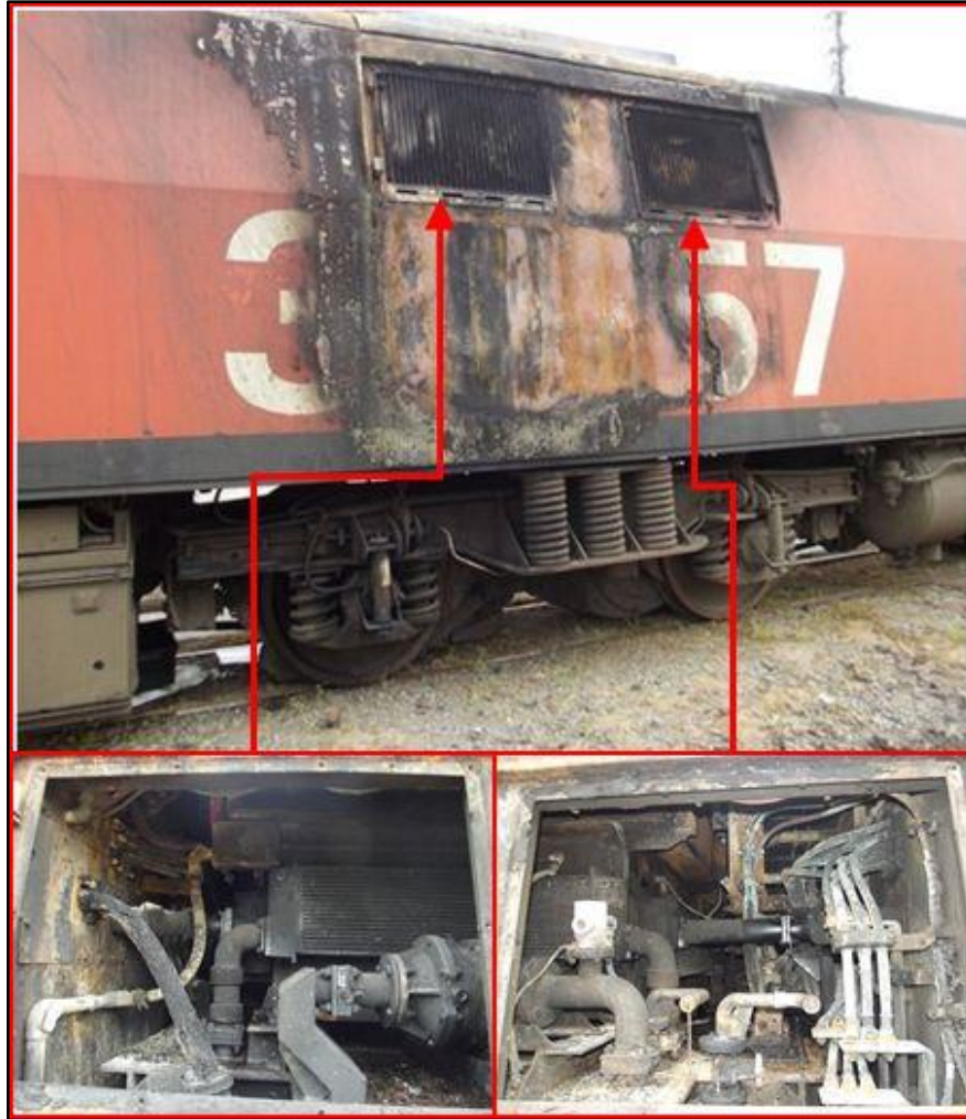
Figure 4 Fire damage to the exterior and interior of the transformer compartment
