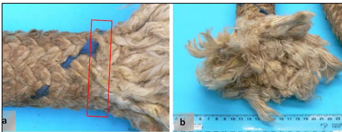
Figure 7 Broken end of choker line (Photo courtesy Scrase Metallurgical Solutions)
